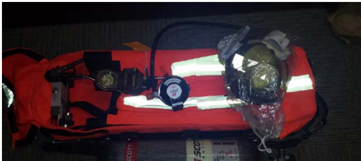
SCOTT_RIT Pack. Rapid Intervention emergency air supply for in-suit emergencies.
