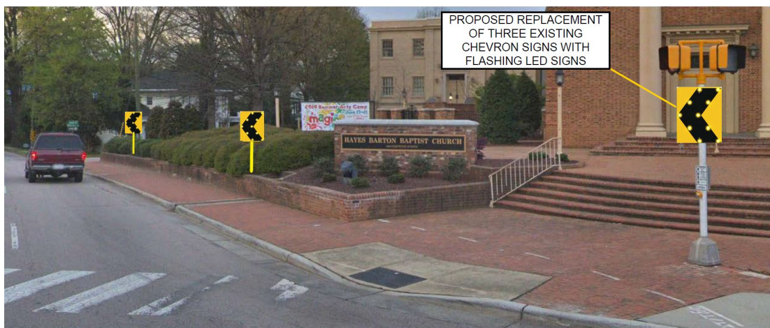
Figure 3 - LED Flashing Chevron Signs – Sketch Plan of Proposed Placement
