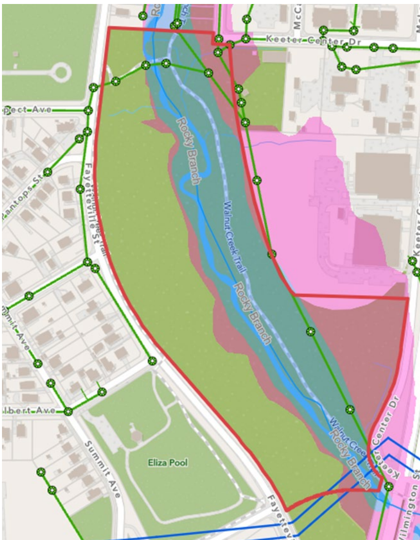
Image showing the extents of the 100 year floodplain extents in the vicinity of 1500 S. Wilmington St (outlined in red). The 500 year elevation adjacent to this property is 243 ft and the 100 year elevation is 236.5 ft.
