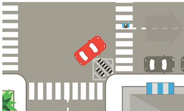
Graphic of vehicle path with turn calming wedge installed
