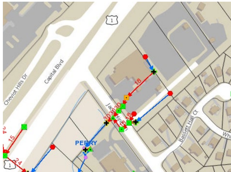
Figure 1. Stormwater pipes on Jacqueline Lane in vicinity of Bassett Hall Court, where reports of street flooding were investigated (note red lines are closed stormwater pipes, blue lines are open stormwater flow channels, green symbols are stormwater catch basins, inlets, and junction boxes).
