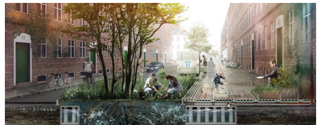
▲ Climate Tile Project in Copenhagen, DK. An example of how streets or "green fingers" that abut a floodplain area can incorporate permeable surfaces that capture/filter excess water and help naturally recharge aquifers. http://theconversation.com
