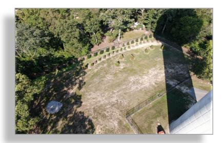
The above "after" picture shows a swale that has been constructed to direct sheet flow from the site to a catch basin, which drains through a pipe to the front of the site along Sunnybrook Road. The additional vegetative plantings are planted along the swale to provide additional visual screening and soften the view for the neighbors.
