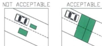
Do not allow the edges of patches to fall in wheel paths.
