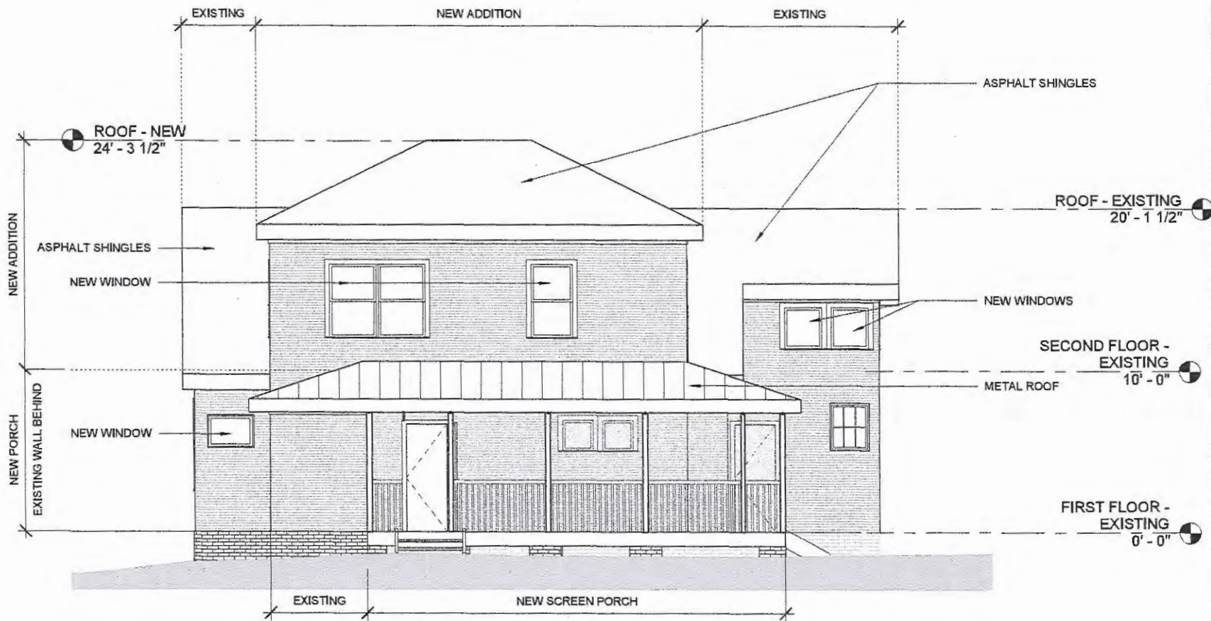
① ELEVATION - SOUTH- RENOVATION 3/16" = 1'-0"
