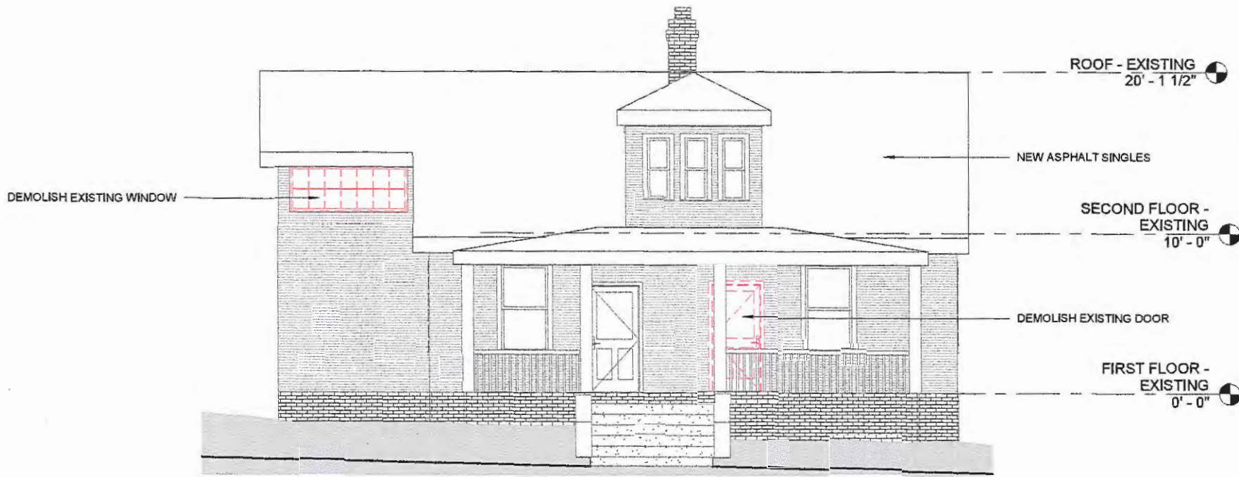
① ELEVATION - NORTH - DEMOLITION 3/16" = 1'-0"
