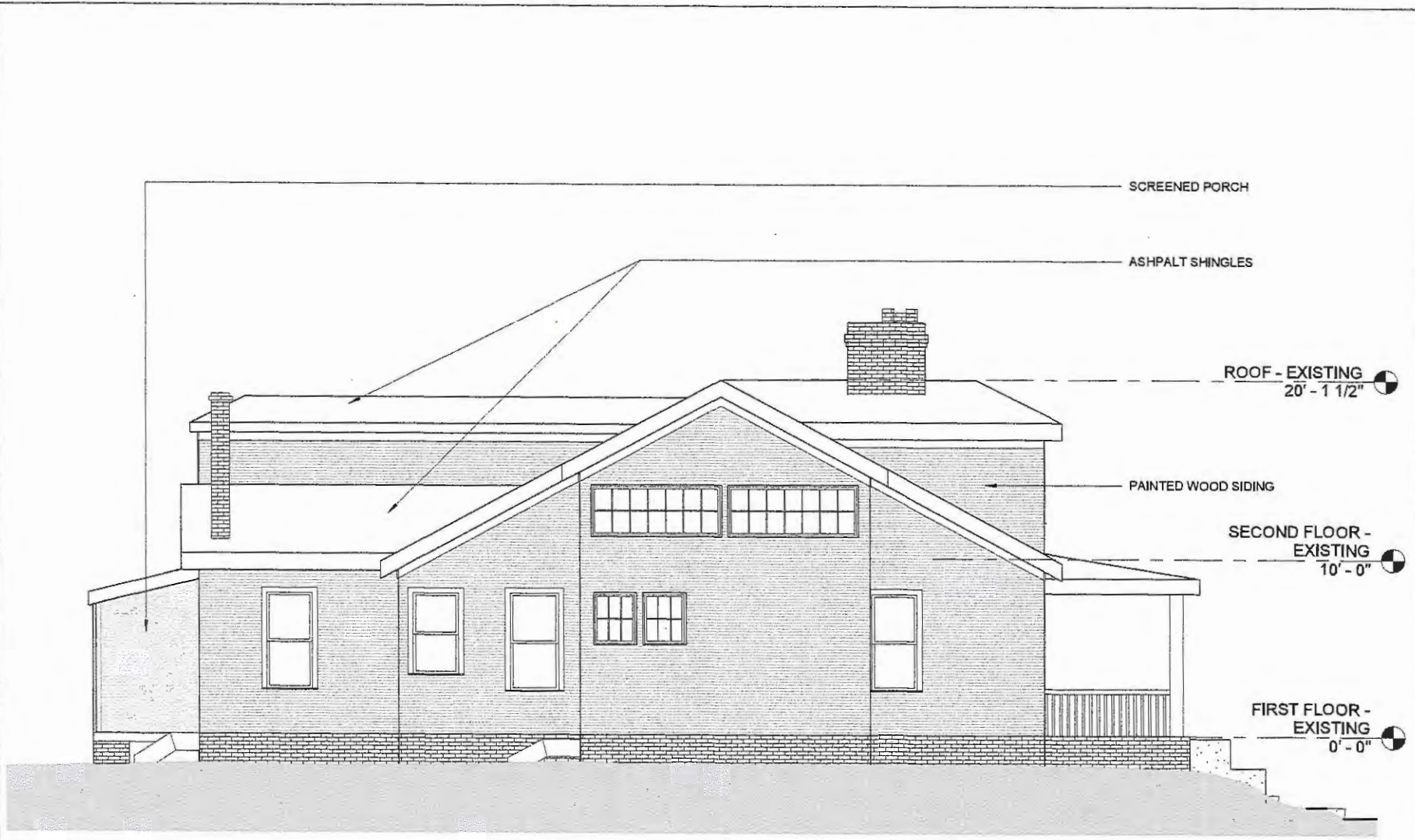
① ELEVATION - EAST-EXISTING 3/16" = 1'-0"
