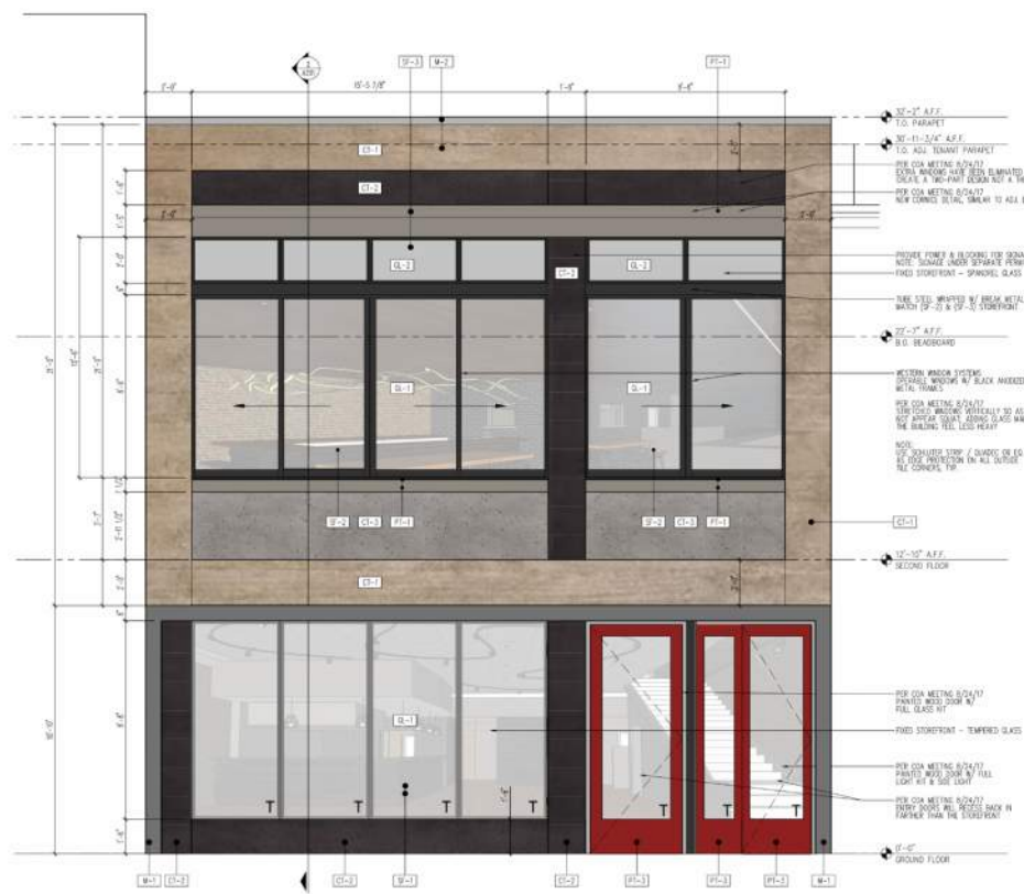
1 Revised Exterior Elevation per COA Meeting 8/24/17 East A201 SCALE: 3/8"=1'-0"
