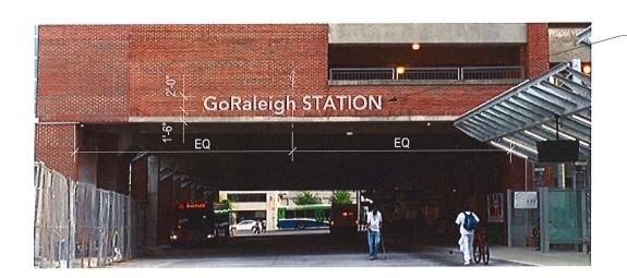
24" HIGH STAINLESS STEEL FABRICATED LETTERS WITH 1 1/2" RETURN - STUD MOUNT TO WALL
