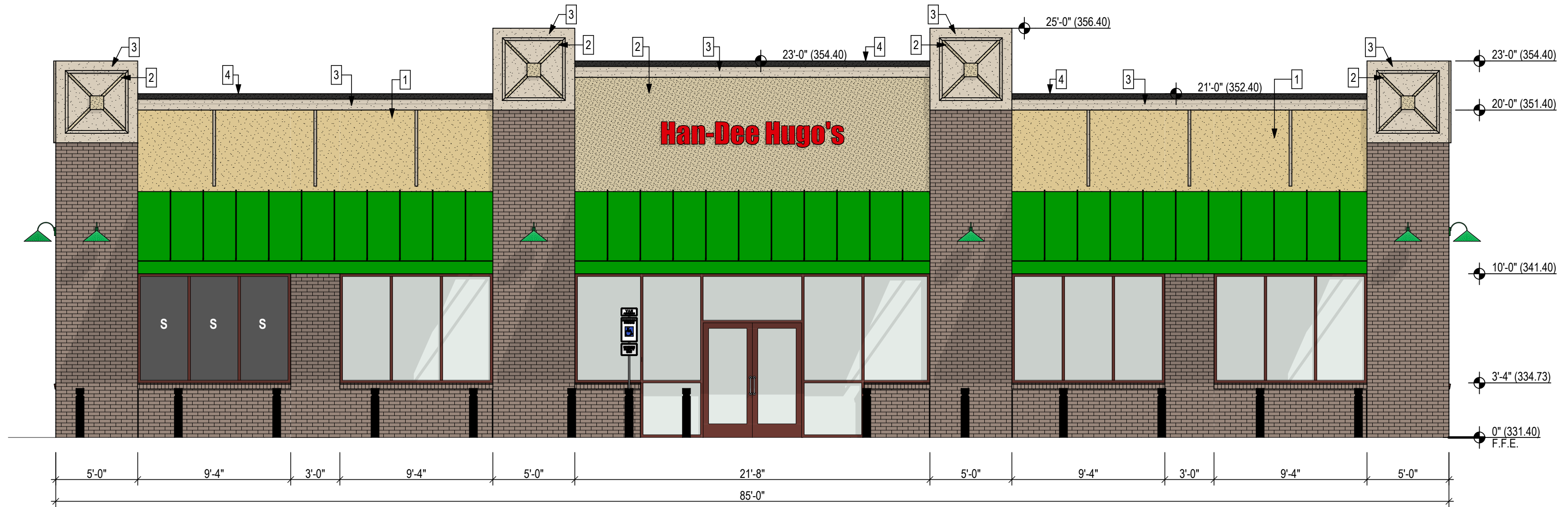
1 WEST ELEVATION NO WINDOWS REQUIRED THIS ELEVATION PER THE UDO, THE DARK GLASS IS SPANDREL GLASS = S SCALE: 3/16" = 1'-0"
