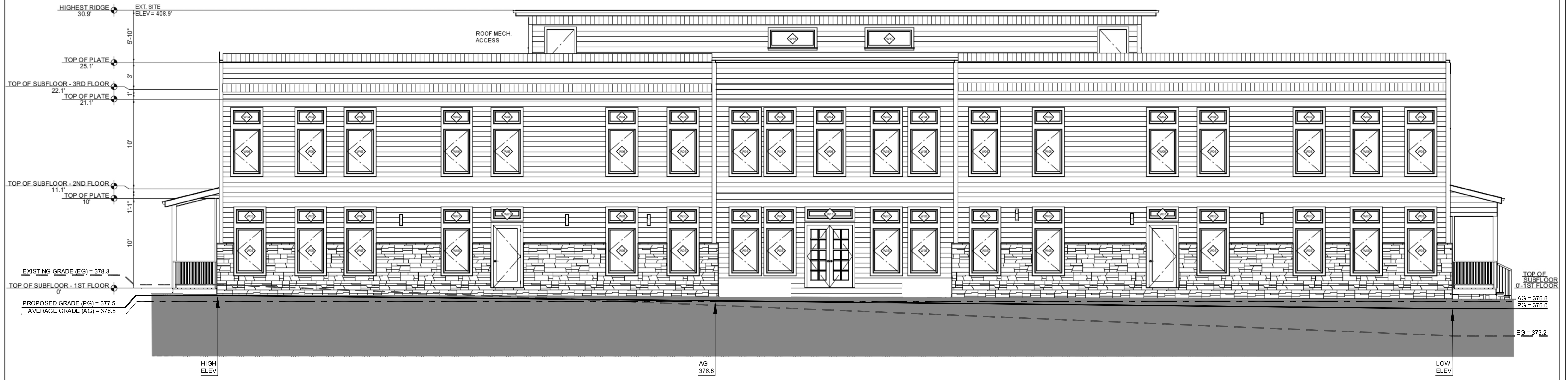
Exterior Elevation Front
