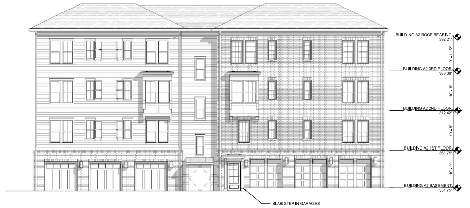
BUILDING A2 - NORTH ELEVATION 2 1/8" = 1'-0"
