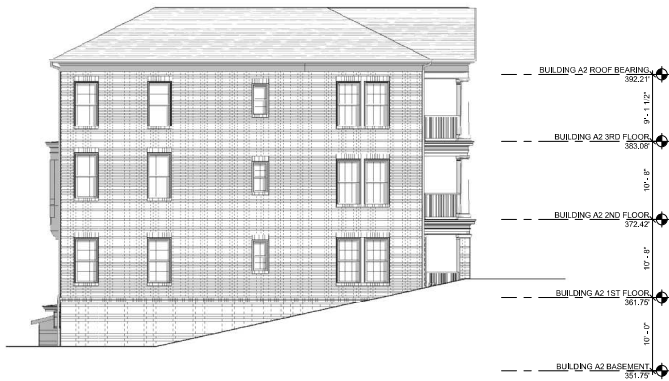
BUILDING A2 - WEST ELEVATION 3 1/8" = 1'-0"
