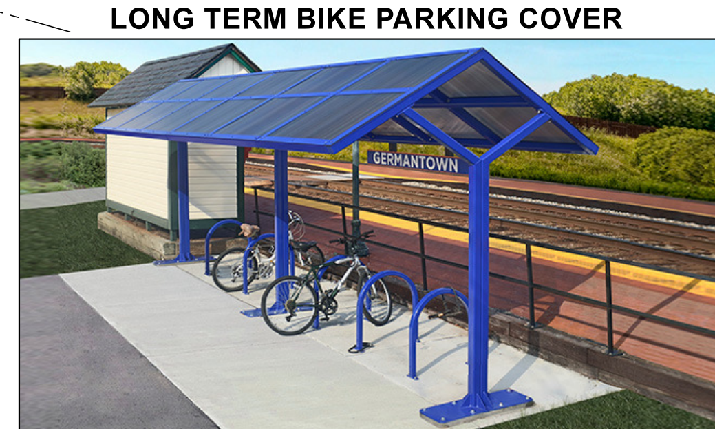
VELODOME SHELTERS MODEL RIDGEFIELD - SINGLE, PAINTED "JET BLACK" 12'L x 9'W x 9'11"H, www.velodomeshelters.com/ridgefield.html
