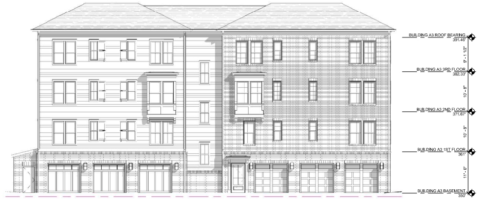
BUILDING A3 - NORTH ELEVATION 2 1/8" = 1'-0"
