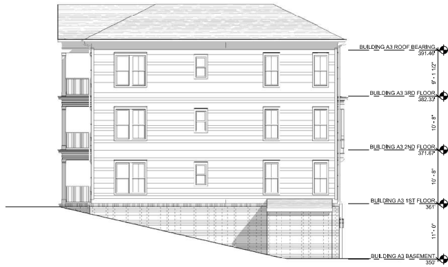
BUILDING A3 - EAST ELEVATION 4 1/8" = 1'-0"
