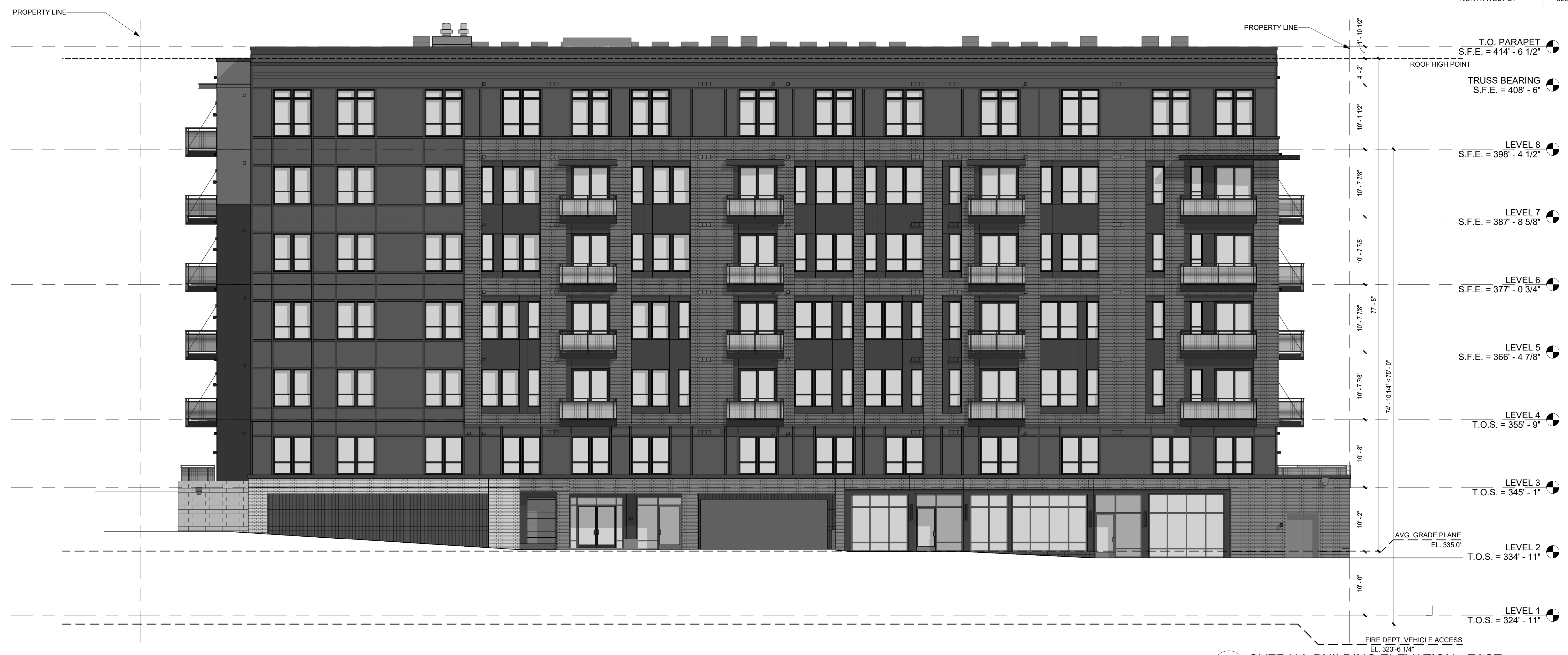
1 OVERALL BUILDING ELEVATION - EAST 1/8" = 1'-0"
