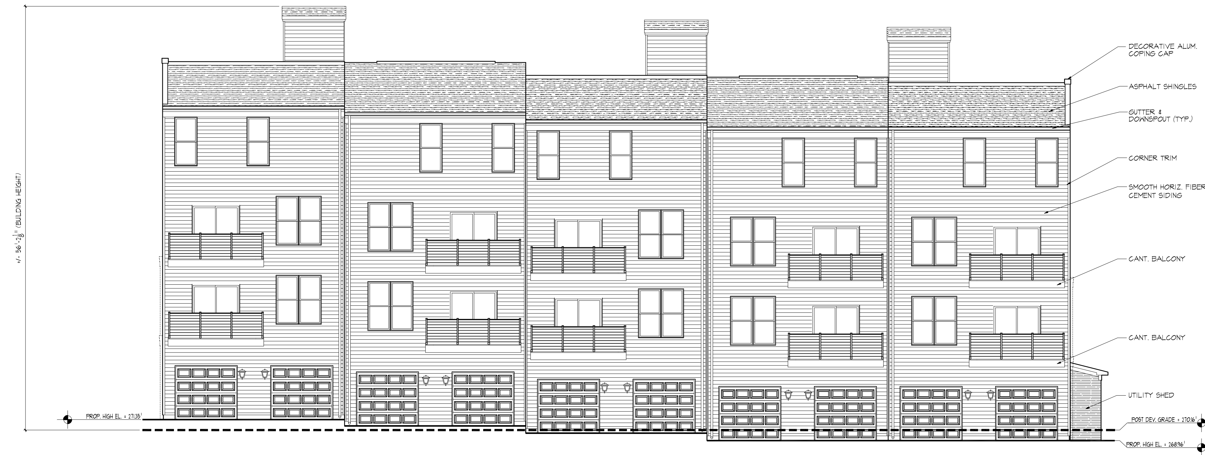
B WEST ELEVATION - BUILDING #7 SCALE 1/8" = 1'-0"
