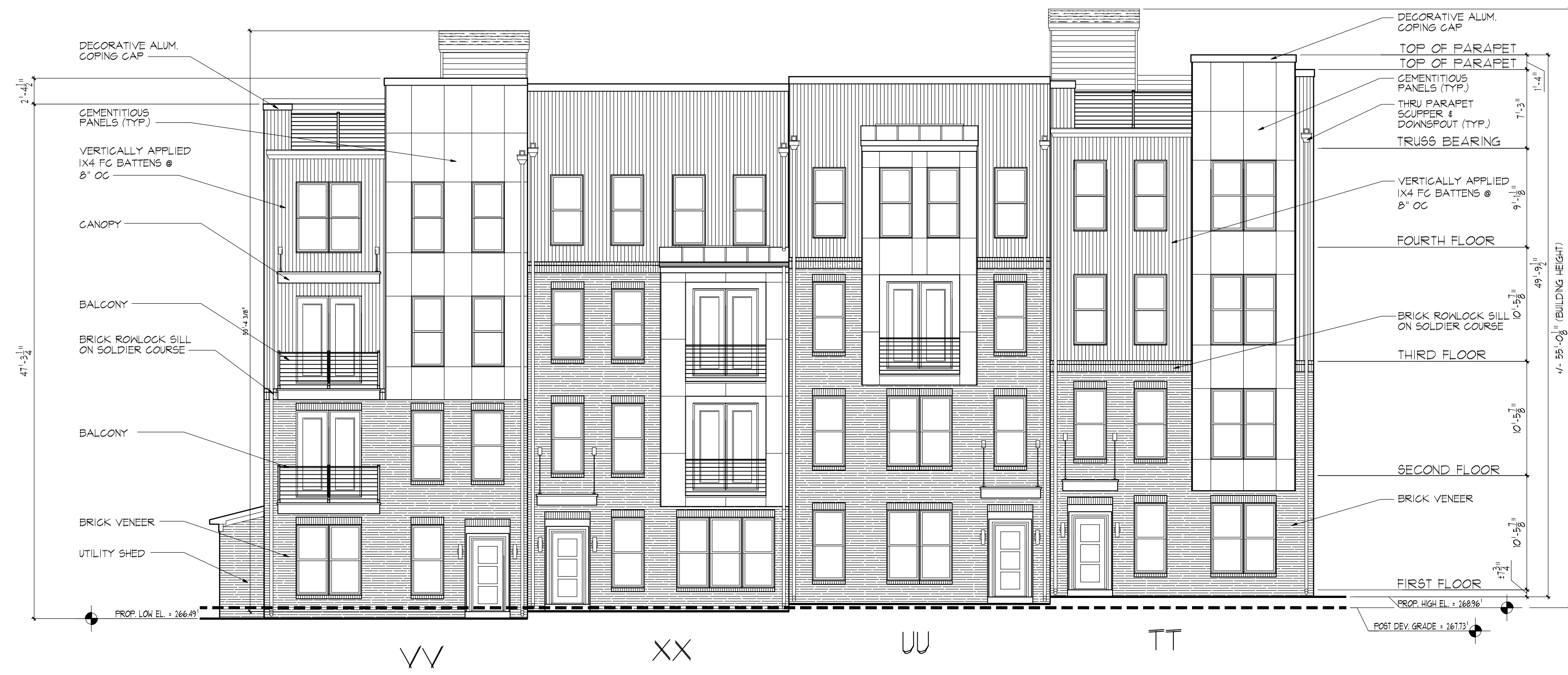
A EAST ELEVATION - BUILDING #8 SCALE 1/8" = 1'-0"
