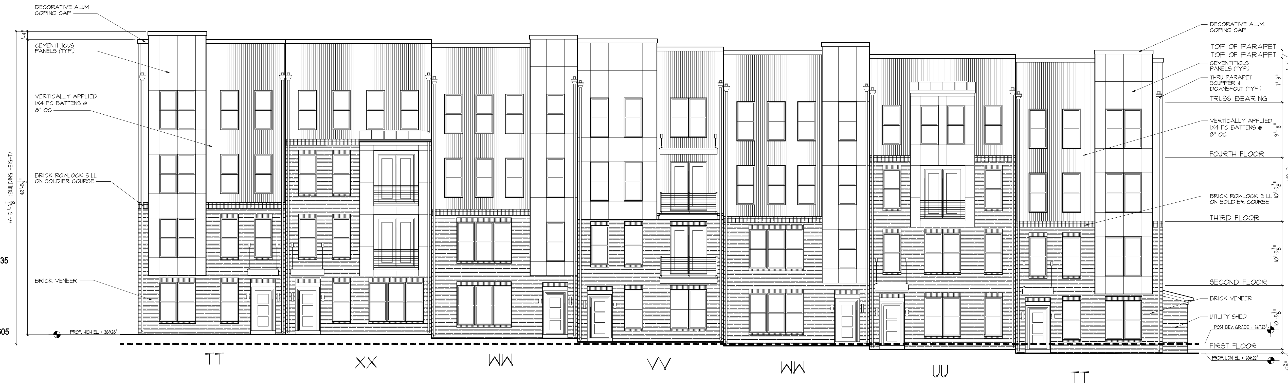
A WEST ELEVATION - BUILDING #9 SCALE 1/8" = 1'-0"
