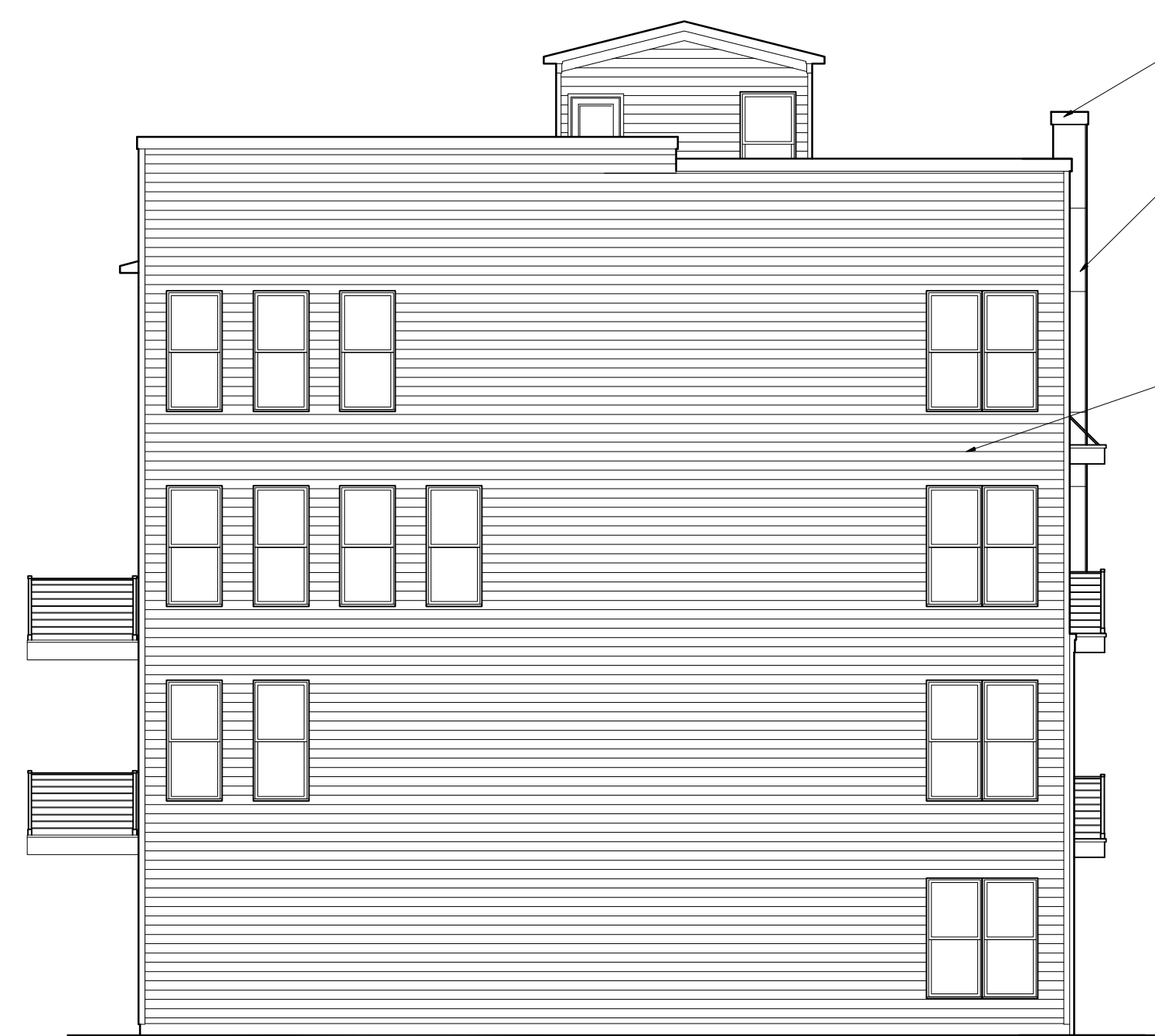
C NORTH ELEVATION - BUILDING #3 A3.0 SCALE 1/8" = 1'-0"
