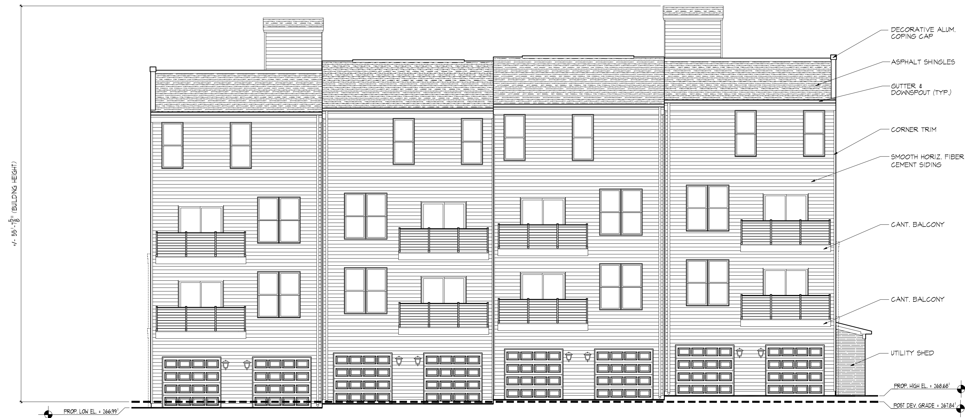
B WEST ELEVATION - BUILDING #8 SCALE 1/8" = 1'-0"
