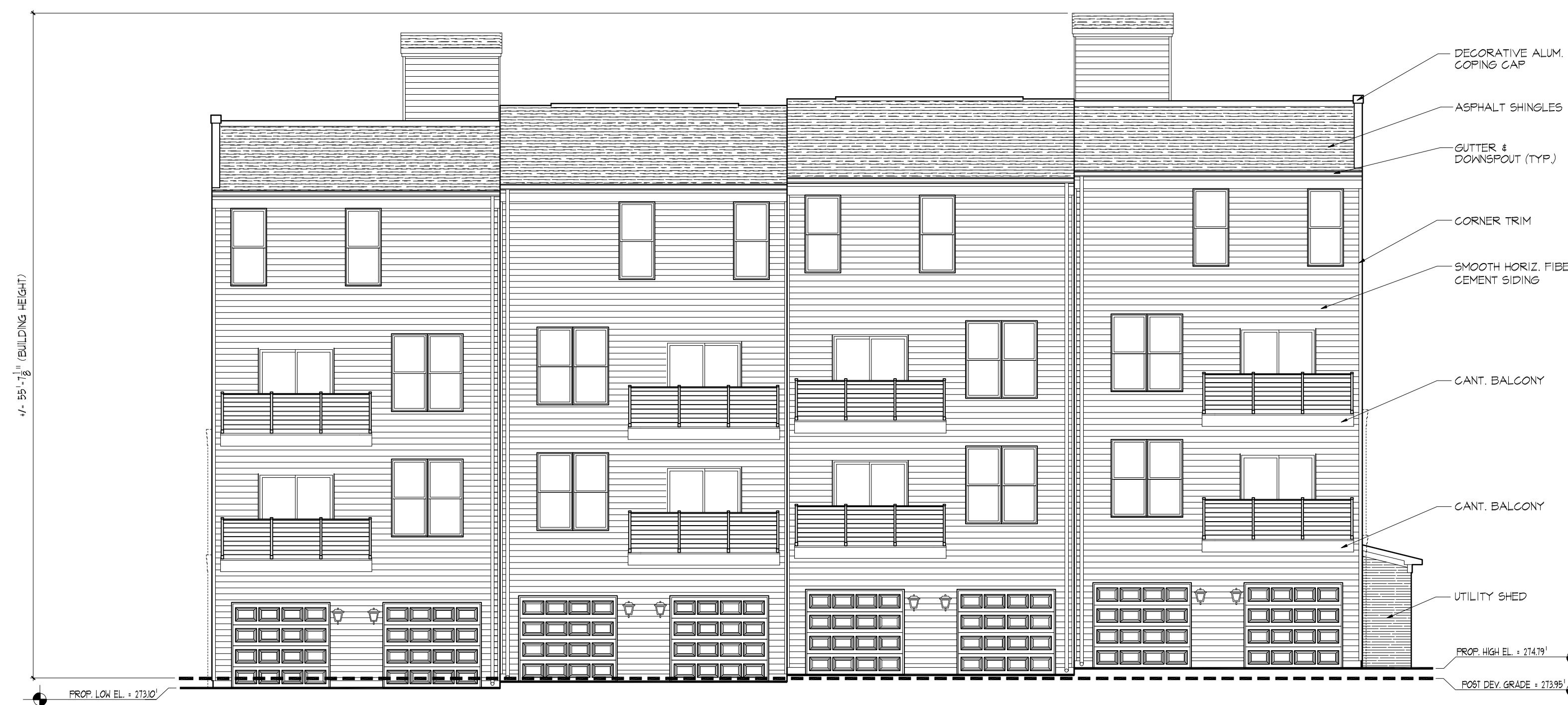
B EAST ELEVATION - BUILDING #5 SCALE 1/8" = 1'-0"
