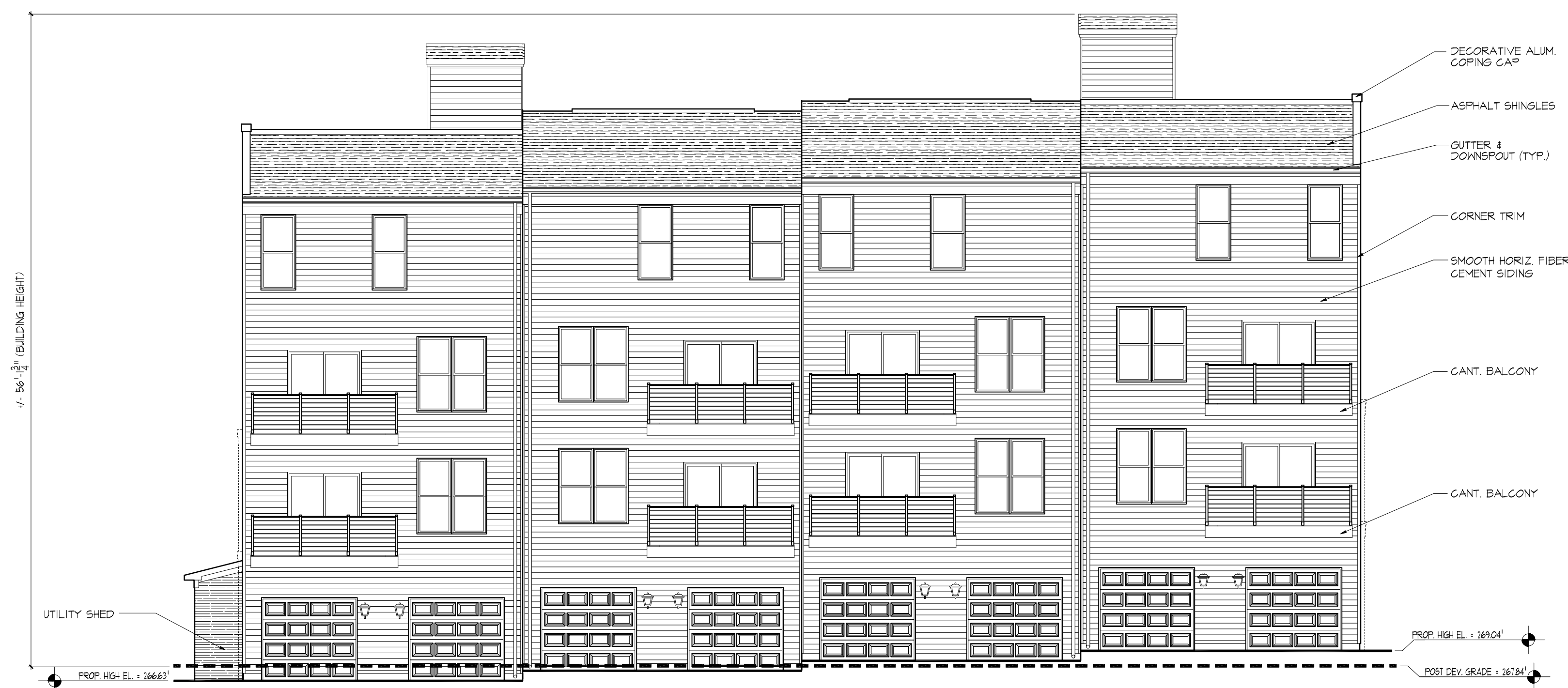
B EAST ELEVATION - BUILDING #3 SCALE 1/8" = 1'-0"
