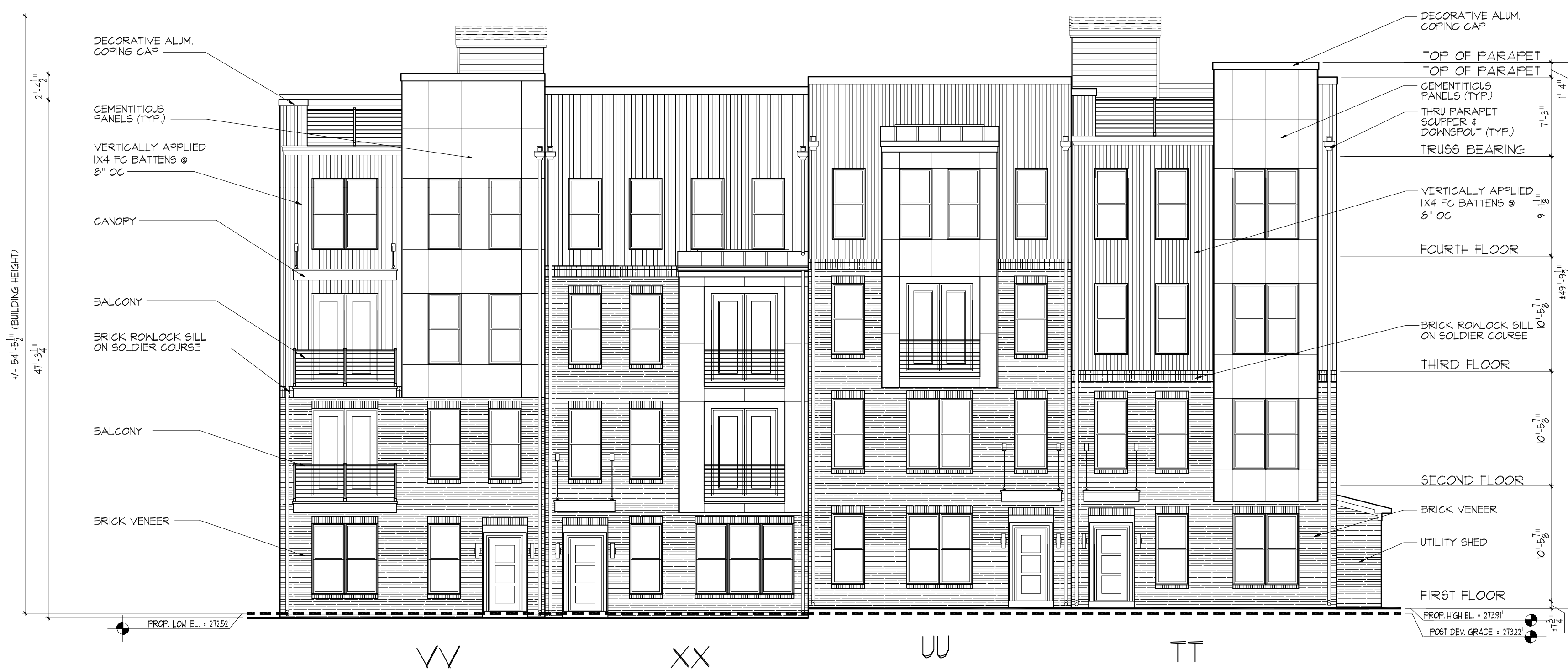
A EAST ELEVATION - BUILDING #6 SCALE 1/8" = 1'-0"
