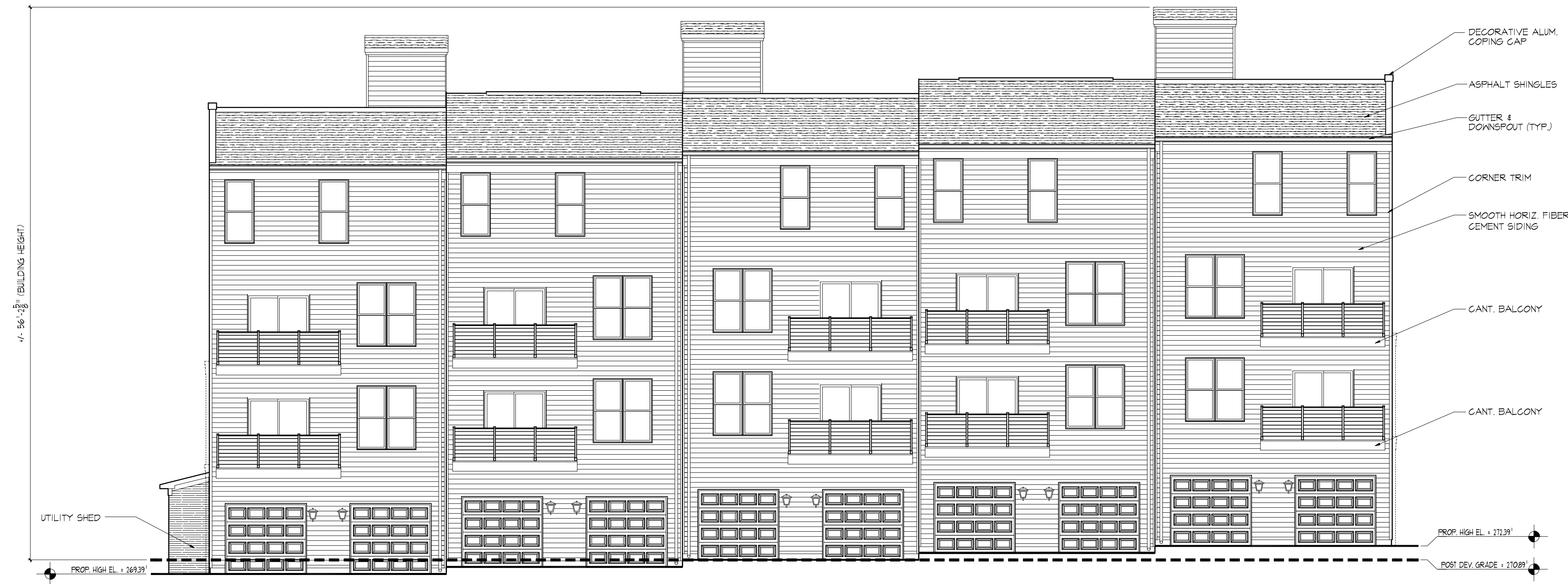
B EAST ELEVATION - BUILDING #4 SCALE 1/8" = 1'-0"
