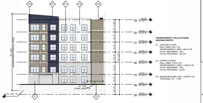
ASR NORTH BLDG. - WEST ELEVATION 1/8" = 1'-0"
