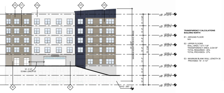
ASR - NORTH BLDG. - NORTH ELEVATION 2 1/8" = 1'-0"
