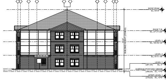
4 WEST BUILDING ELEVATION (PARKING LOT VIEW) A201 3/32" = 1'-0"
