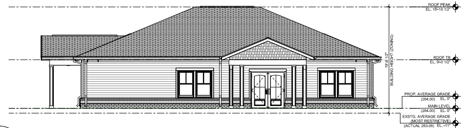
2 NORTH BUILDING ELEVATION A307 3/16" = 1'-0"
