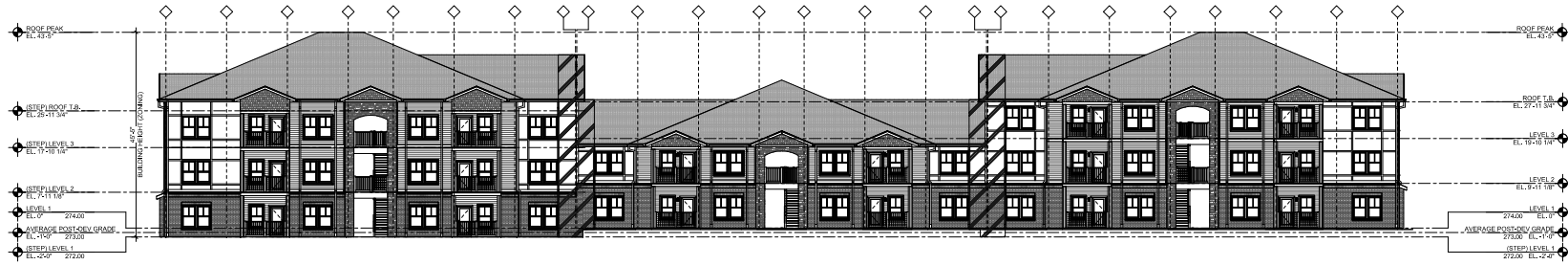
1 WEST BUILDING ELEVATION (PARKING LOT VIEW) 3/32" = 1'-0"
