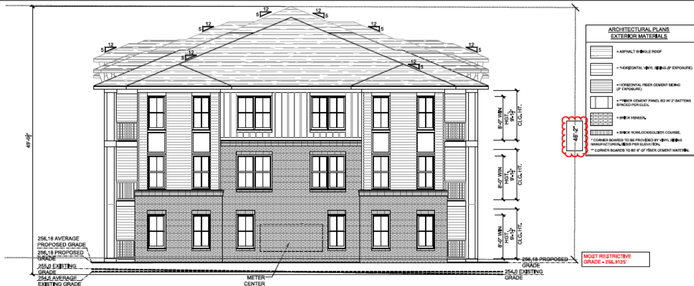
2 SITE BUILDING #1 - TYPE 1 - RIGHT ELEVATION (EAST) Scale: 3/16" = 1'-0"
