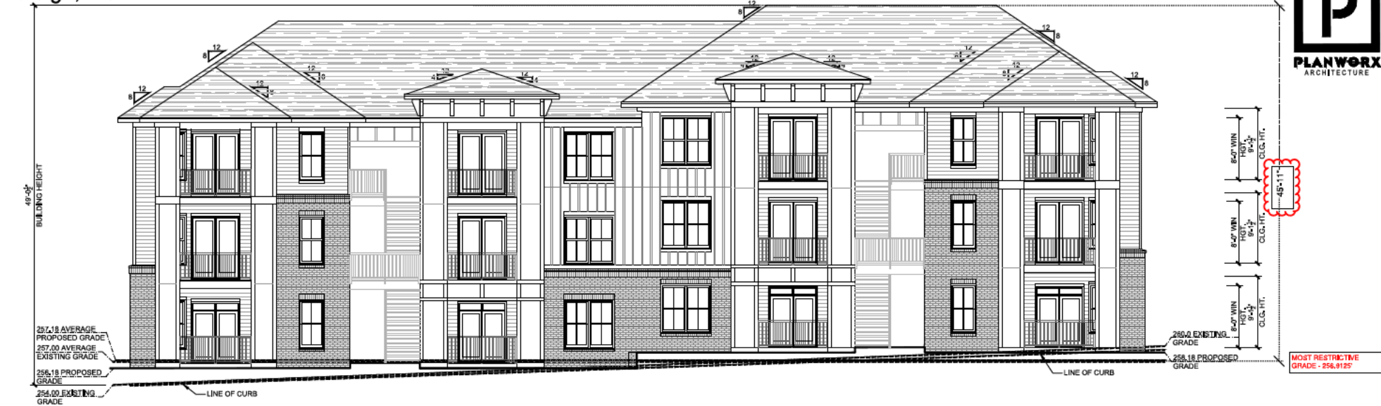
1 SITE BUILDING #1 - TYPE 1 - REAR ELEVATION (NORTH) Scale: 3/16" = 1'-0"
