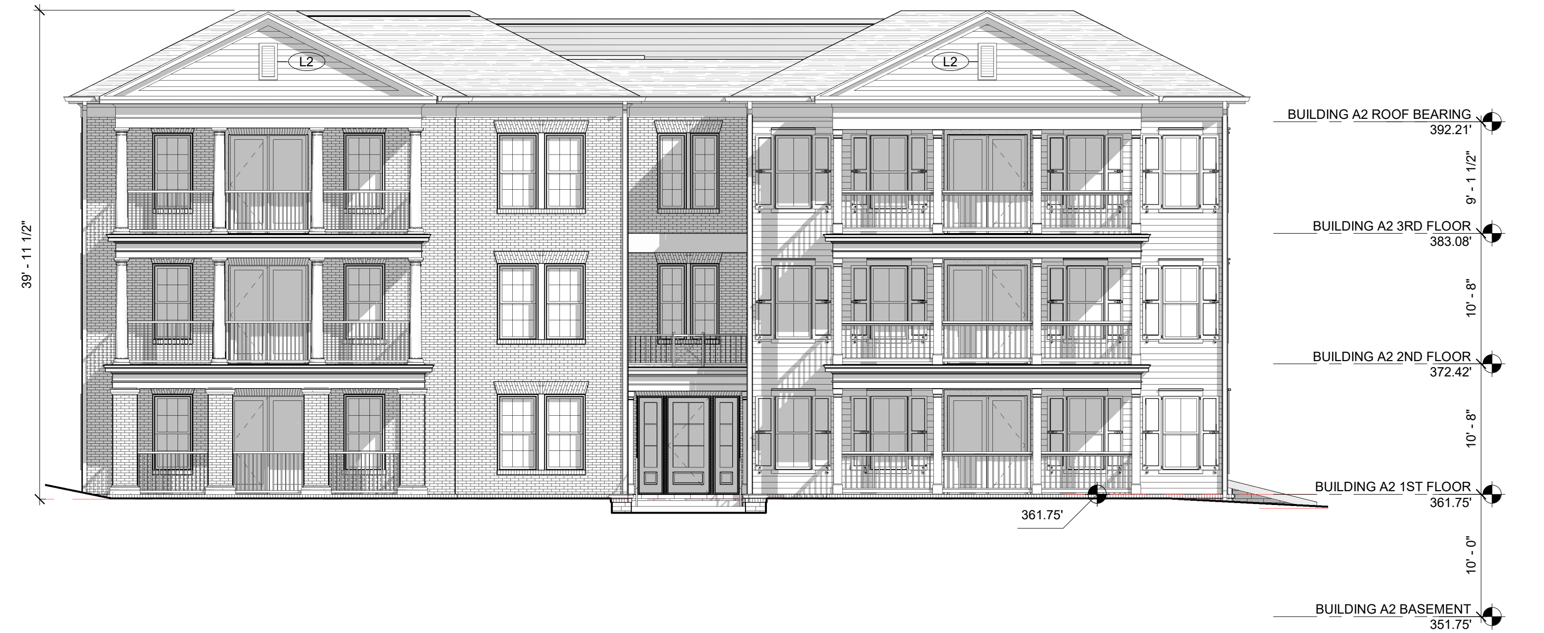
BUILDING A2 - SOUTH ELEVATION ASR 1 1/8" = 1'-0"
