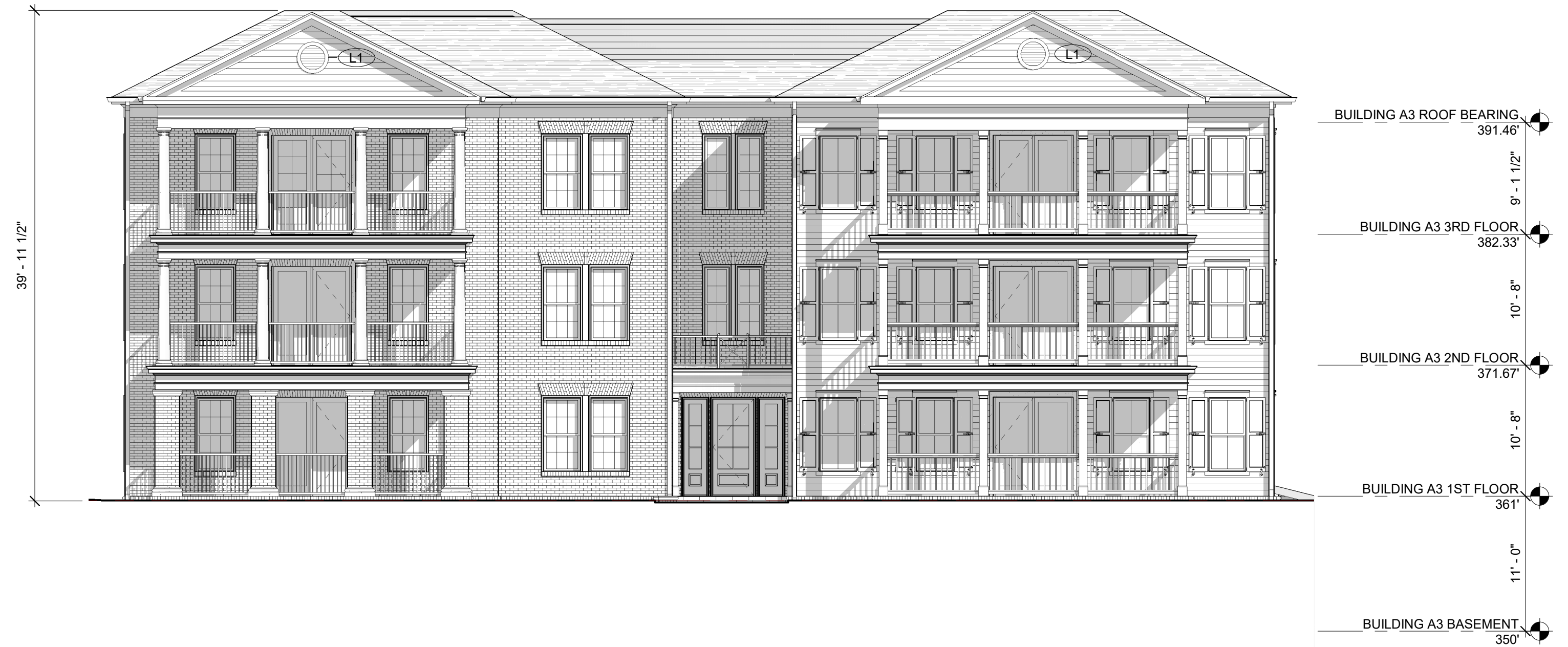
BUILDING A3 - SOUTH ELEVATION ASR 1 1/8" = 1'-0"
