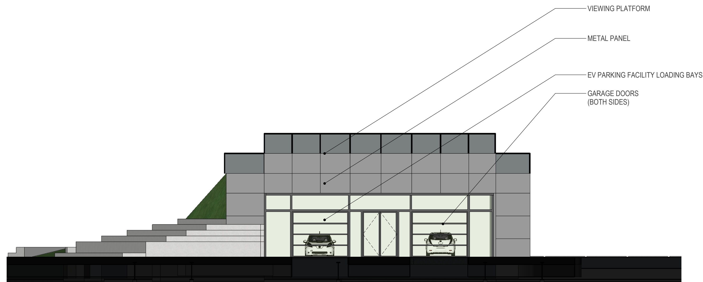
3 NORTH ACCESS LOADING BAY ELEVATION A-205 1/8" = 1'-0"
