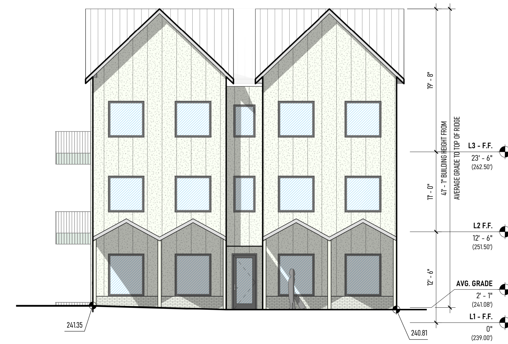
1 1113 BROOKSIDE - EAST ENTRANCE ELEVATION 1/8" = 1'-0"
