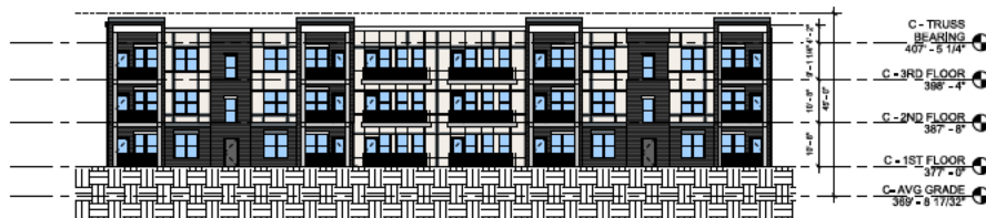
4 BLDG C - WEST ELEVATION 1/16" = 1'-0"
