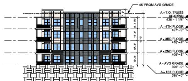
3 BLDG A - EAST ELEVATION 1/16" = 1'-0"
