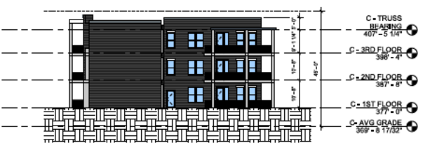
2 BLDG C - SOUTH ELEVATION 1/16" = 1'-0"
