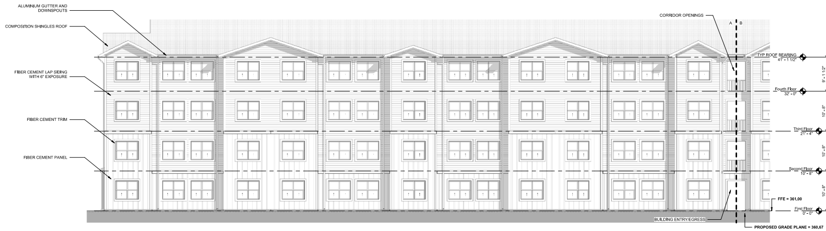
BUILDING 5 ASR ELEVATION - NORTH A 1 1/8" = 1'-0"
