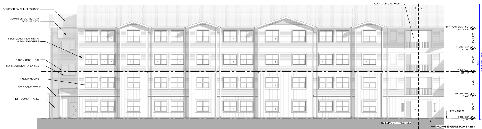
BUILDING 4 ASR ELEVATION - NORTH B 2 1/8" = 1'-0"
