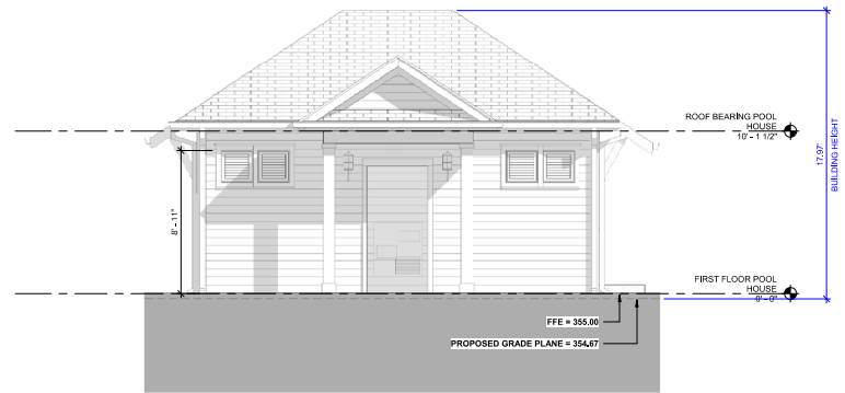
POOLHOUSE ELEVATION - NORTH 1 1/4" = 1'-0"
