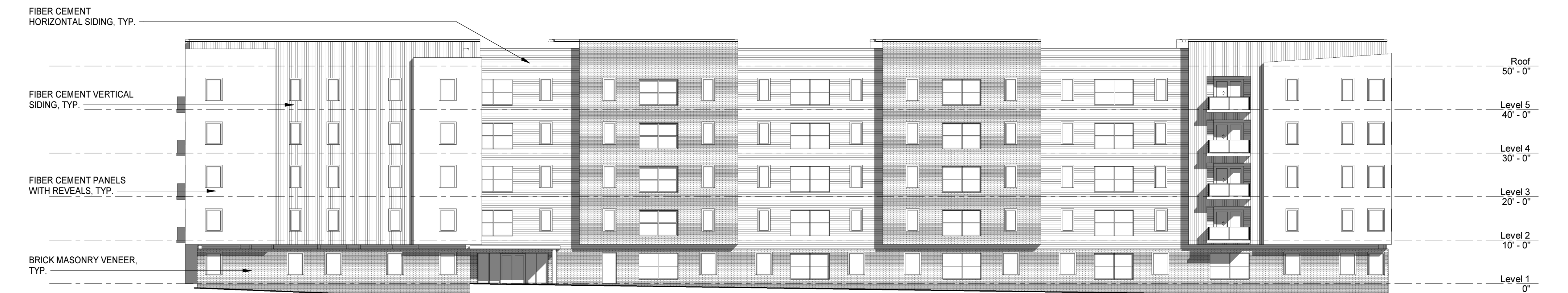
3 BUILDING A SOUTH ELEVATION A2.1.1 | A4.1.1 | 1/16" = 1'-0"
