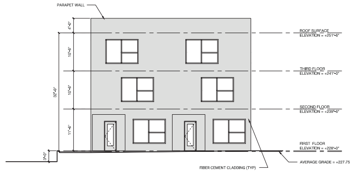
3 NORTH ELEVATION "C" SCALE = 1/8" = 1'-0"
