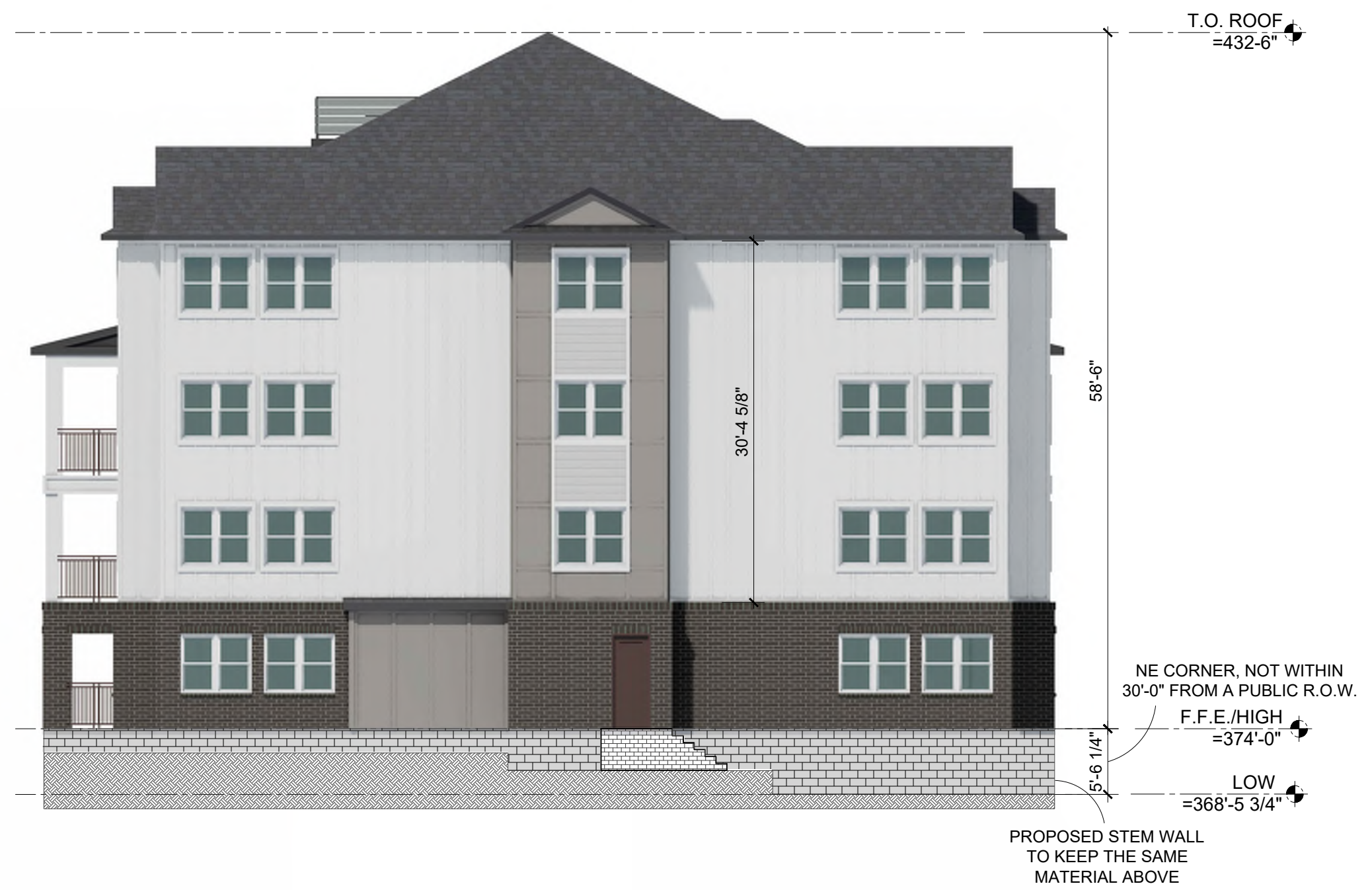
04 BUILDING #1 (TYPE I) - SIDE ELEVATION SCALE: 3/32" = 1'-0" EAST
