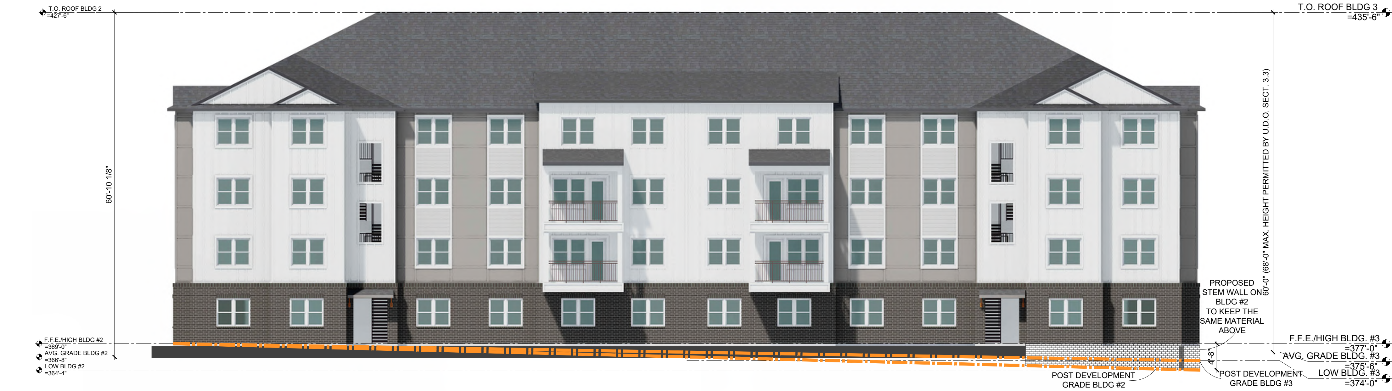
01 BUILDING #2, #3 (TYPE II) - FRONT ELEVATION SCALE: 3/32" = 1'-0" SIDE FACING PRIMARY STREET - SOUTH
