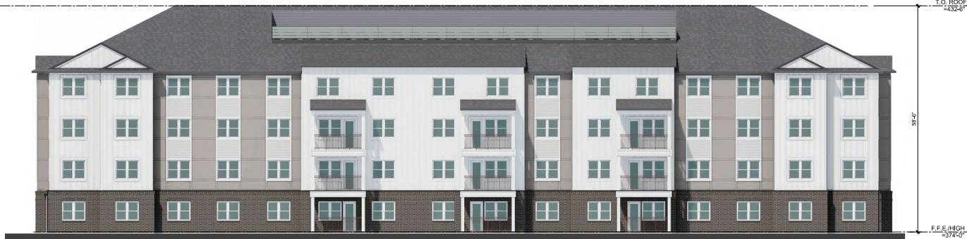
02 BUILDING #1 (TYPE I) - REAR ELEVATION SCALE: 3/32" = 1'-0" SOUTH
