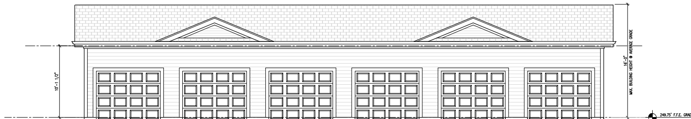
6 CAR GARAGE- G8 - FRONT ELEVATION SCALE: 1/4" = 1'-0"
