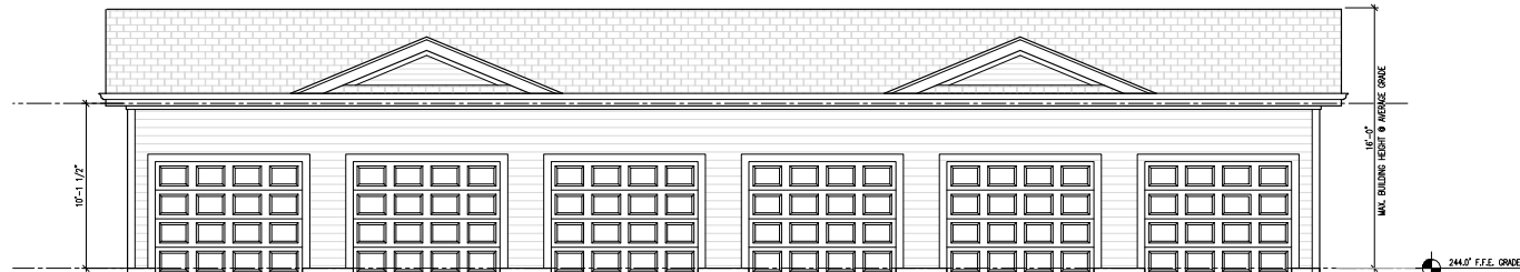
6 CAR GARAGE- G5 - FRONT ELEVATION SCALE: 1/4" = 1'-0"
