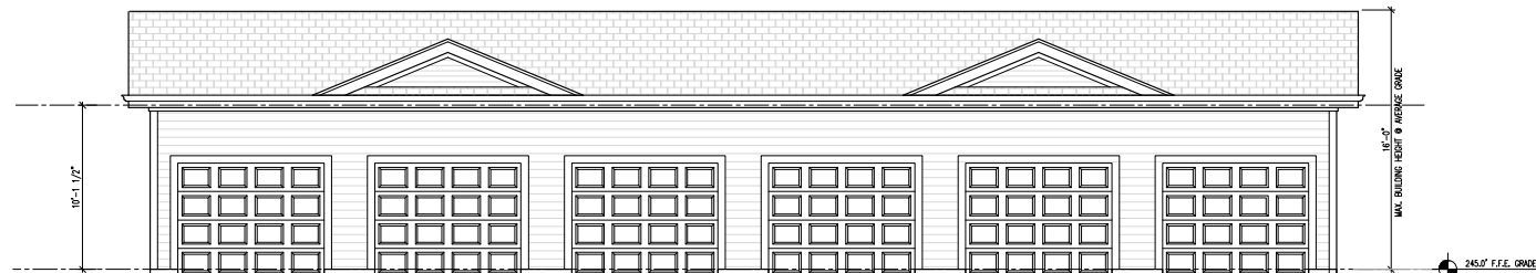
6 CAR GARAGE- G4 - FRONT ELEVATION SCALE: 1/4" = 1'-0"
