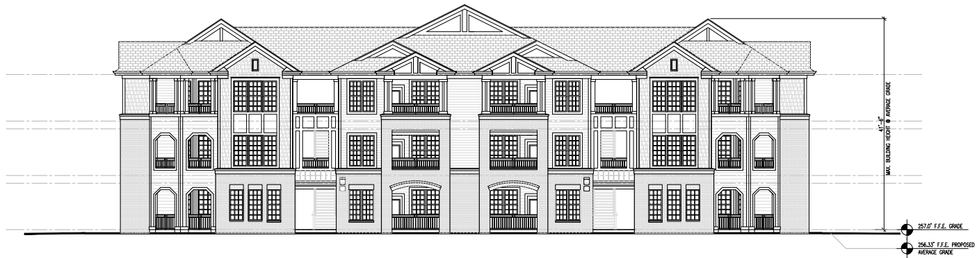
BUILDING TYPE 9 - FRONT ELEVATION (BUILDING #1) SCALE: 1/8" = 1'-0"
