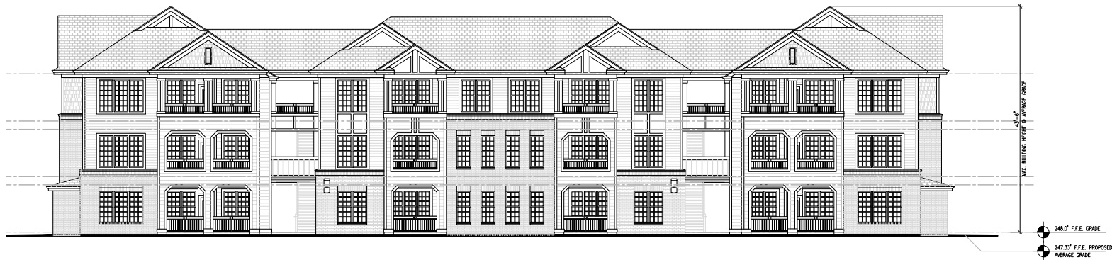
BUILDING TYPE 3 - FRONT ELEVATION (BUILDING #13) SCALE: 1/8" = 1'-0"
