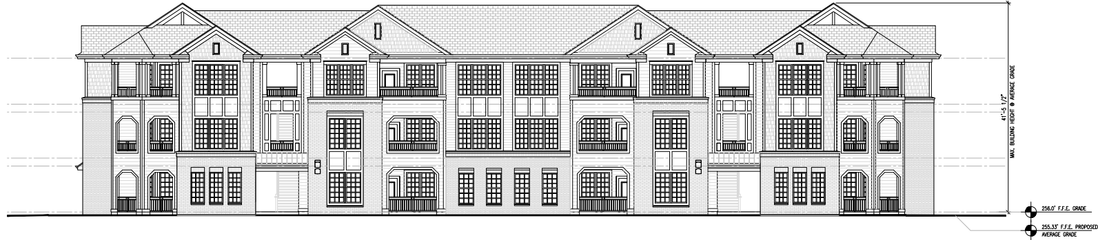
BUILDING TYPE 4 - FRONT ELEVATION (BUILDING #8) SCALE: 1/8" = 1'-0"
