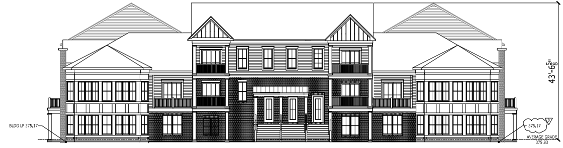
D BUILDING 1 EAST ELEVATION A-2.0 Scale: 1/8" = 1'-0"
