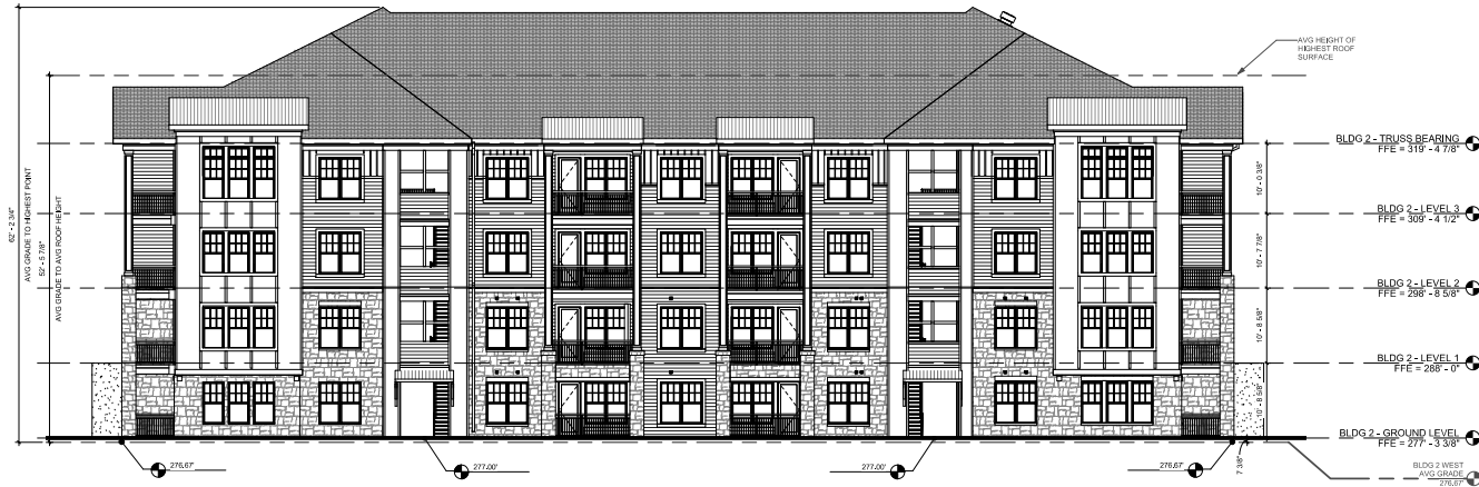
2 BLDG 2000 OVERALL WEST ELEVATION 1/8" = 1'-0" PROPOSED AVERAGE GRADE PLANE WEST ELEVATION = 276.67'
