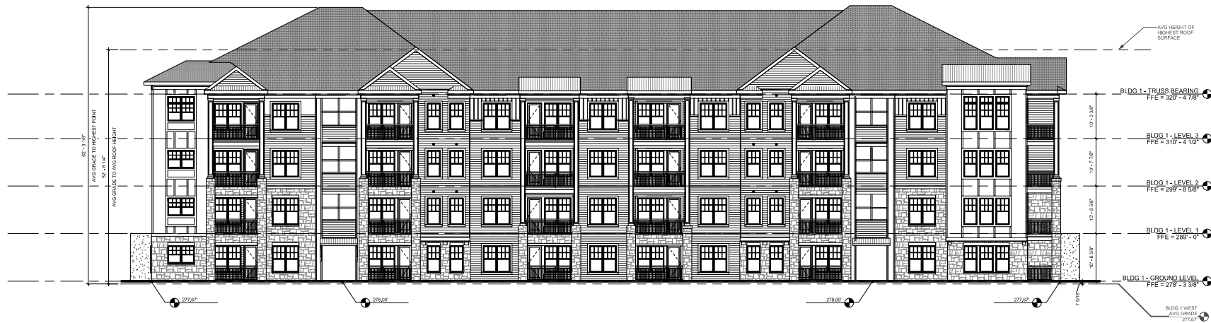
2 BLDG 1000 OVERALL WEST ELEVATION 1/8" = 1'-0" PROPOSED AVERAGE GRADE PLANE WEST ELEVATION - 277.67'
