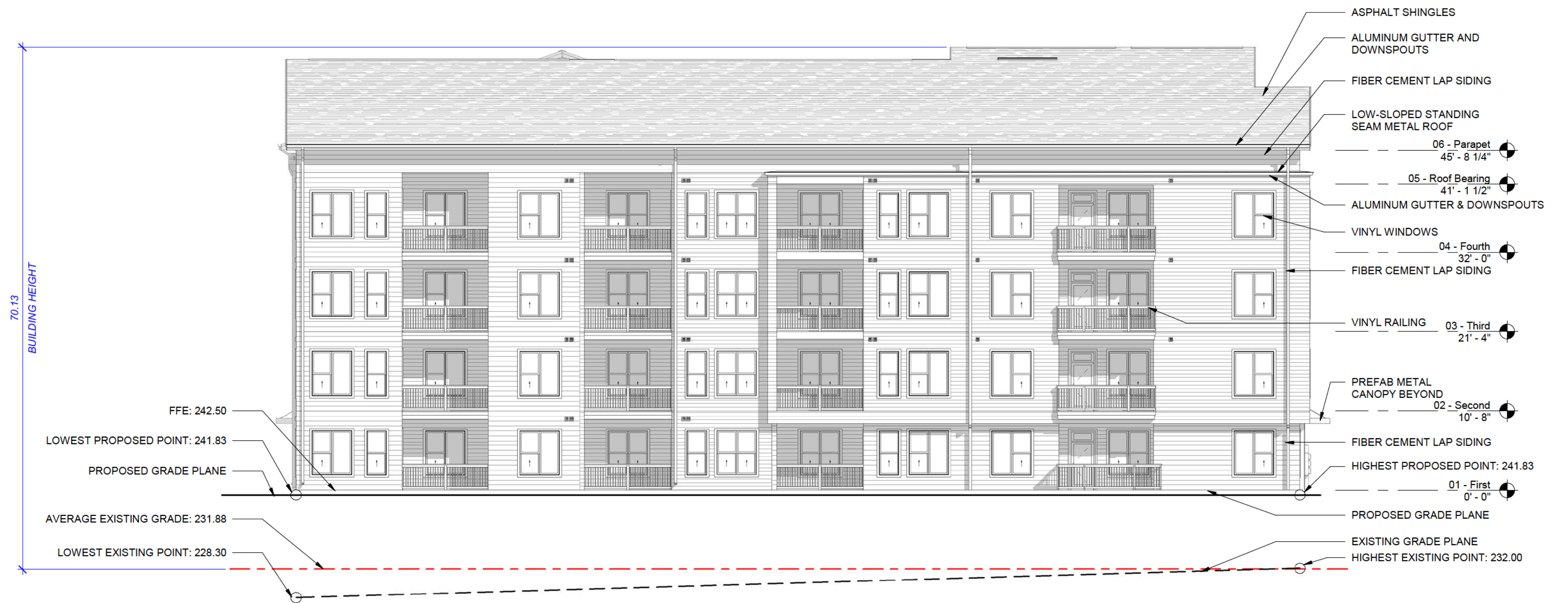
BUILDING 4 - EAST ELEVATION 2 3/32" = 1'-0"
