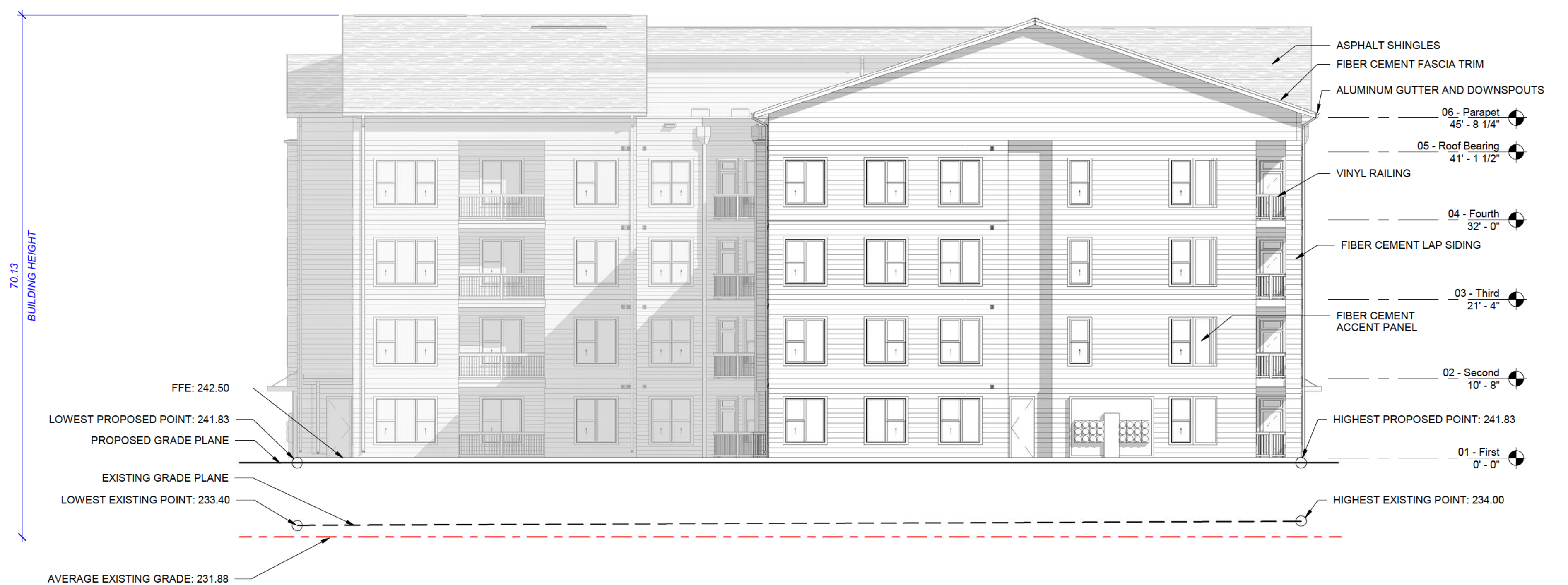
ASR 15 BLDG 4 - WEST ELEVATION 1 3/32" = 1'-0"
