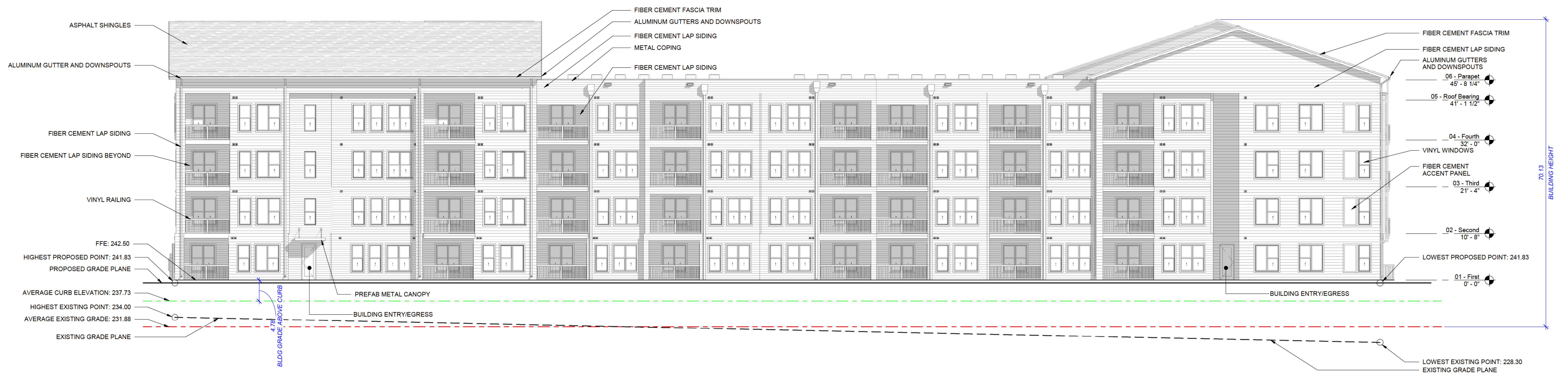
BUILDING 4 - SOUTH ELEVATION (ALLOY ST.) 1 3/32" = 1'-0"
