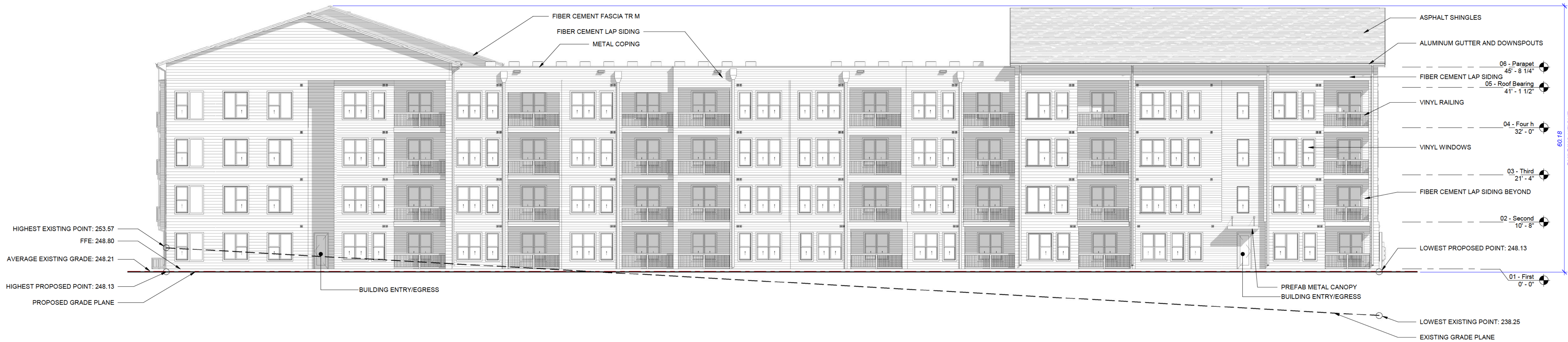
BUILDING 3 - EAST ELEVATION 4 3/32" = 1'-0"
