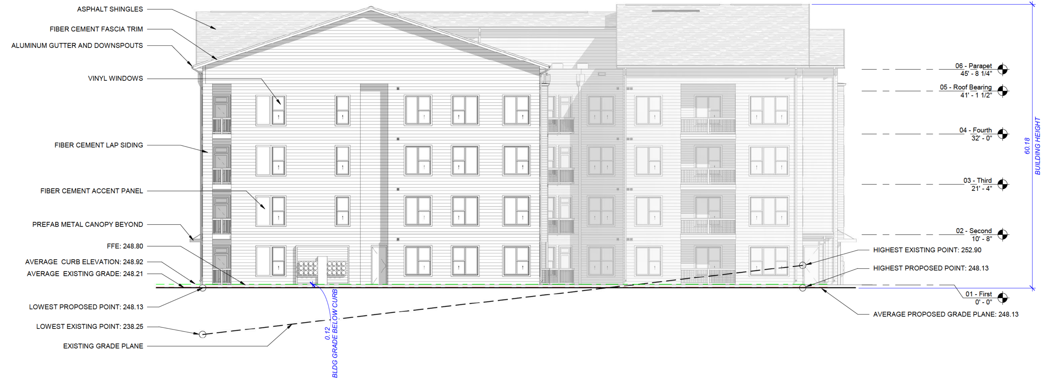
BUILDING 3 - NORTH ELEVATION (ALLOY ST.) 4 3/32" = 1'-0"
