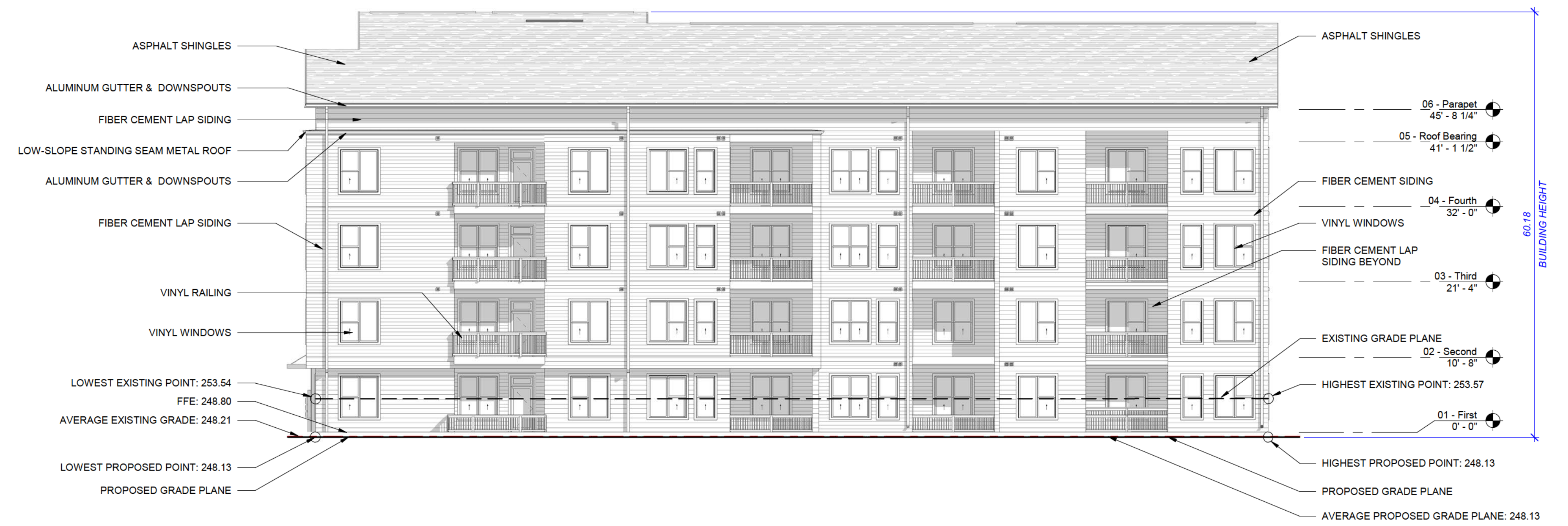
BUILDING 3 - SOUTH ELEVATION 3 3/32" = 1'-0"
