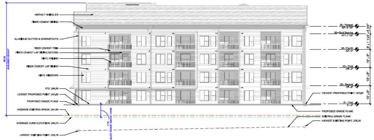
BUILDING 2 - NORTH ELEVATION (ALLOY ST.) 4 3/32" = 1'-0"
