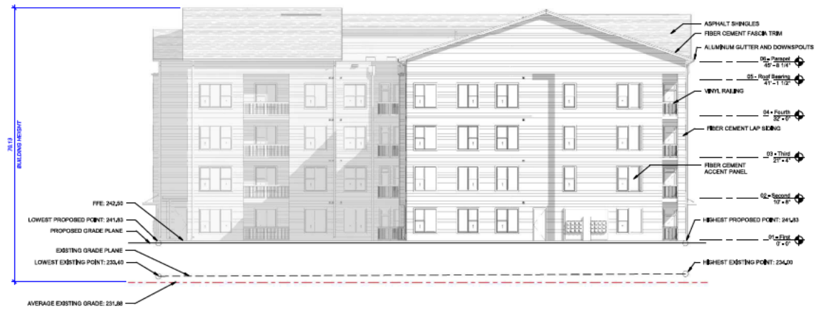
ASR 15 BLDG 4 - WEST ELEVATION 1 3/32" = 1'-0"
