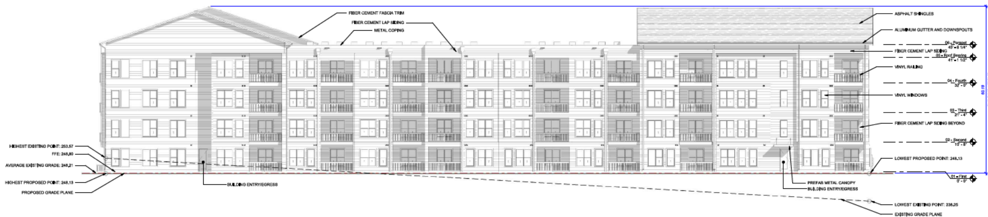
BUILDING 3 - EAST ELEVATION 4 3/32" = 1'-0"
