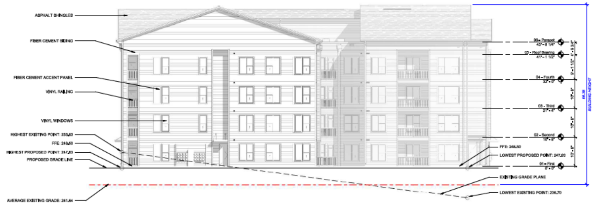
BUILDING 2 - SOUTH ELEVATION 3 3/32" = 1'-0"
