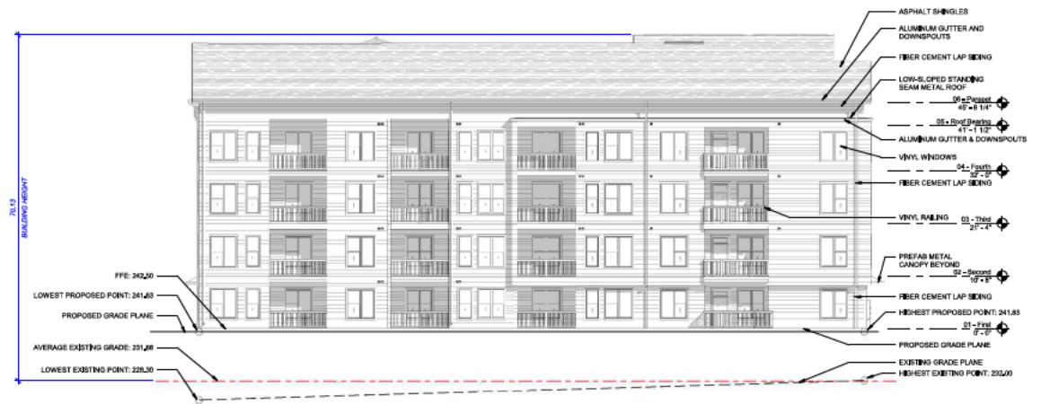
BUILDING 4 - EAST ELEVATION 2 3/32" = 1'-0"
