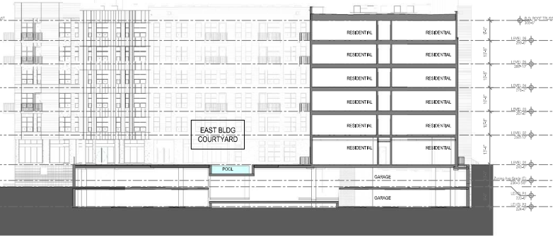
A5 BUILDING SECTION - EAST BLDG (N-S)
