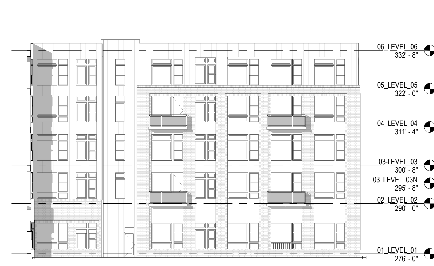
SOUTH COURTYARD - SOUTH ELEVATION 1/16" = 1'-0" 3
