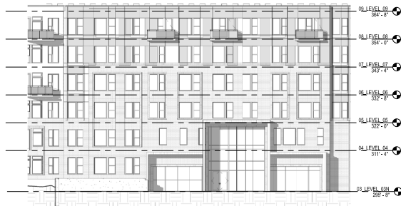
Elevation: North Courtyard (E) Material Area % of Total % of Total w/o Glazing Brick 3197 30.5% 53% Panel 2593 24.8% 43% Glazing 4476 42.7% Metal/Wood 210 2.0% Total 10476
