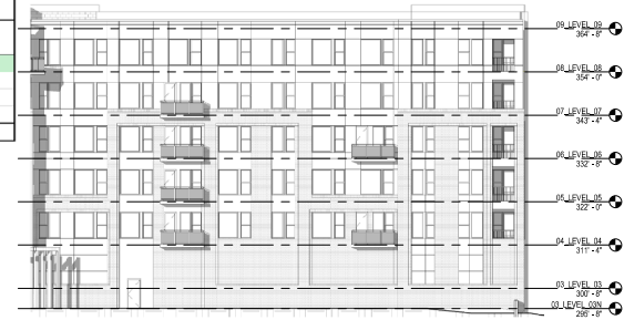
Elevation: North Courtyard (S) Material Area % of Total % of Total w/o Glazing Brick 2680 32.1% 52% Panel 2430 29.1% 48% Glazing 3250 38.9% Metal/Wood 0.0% Total 8360
