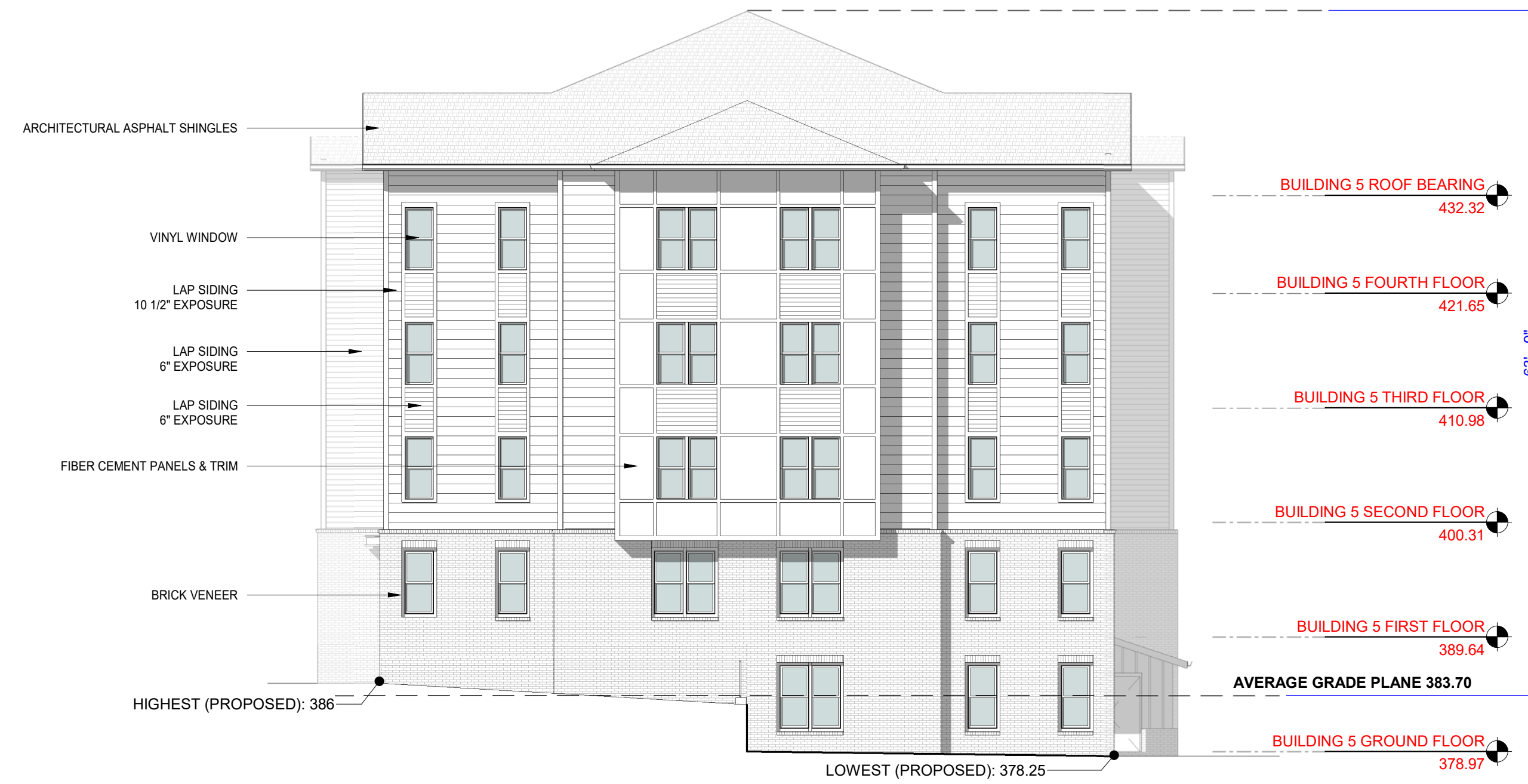
BUILDING 5 - EAST ELEVATION PRIMARY STREET
