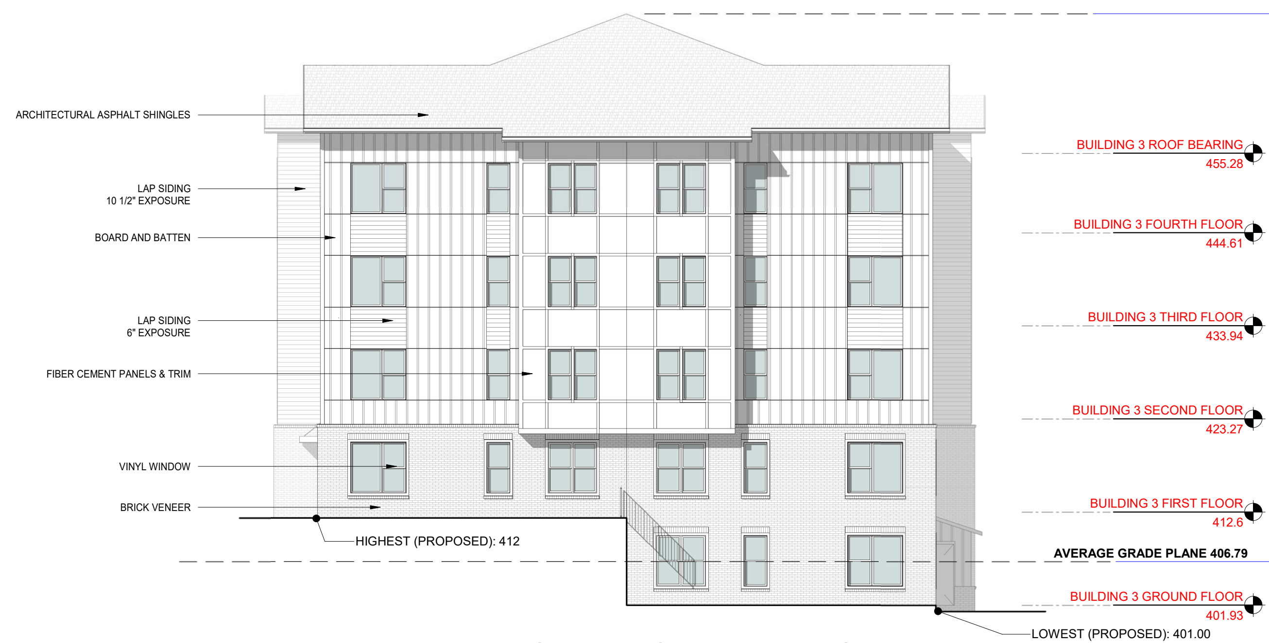
BUILDING 3 - EAST ELEVATION
