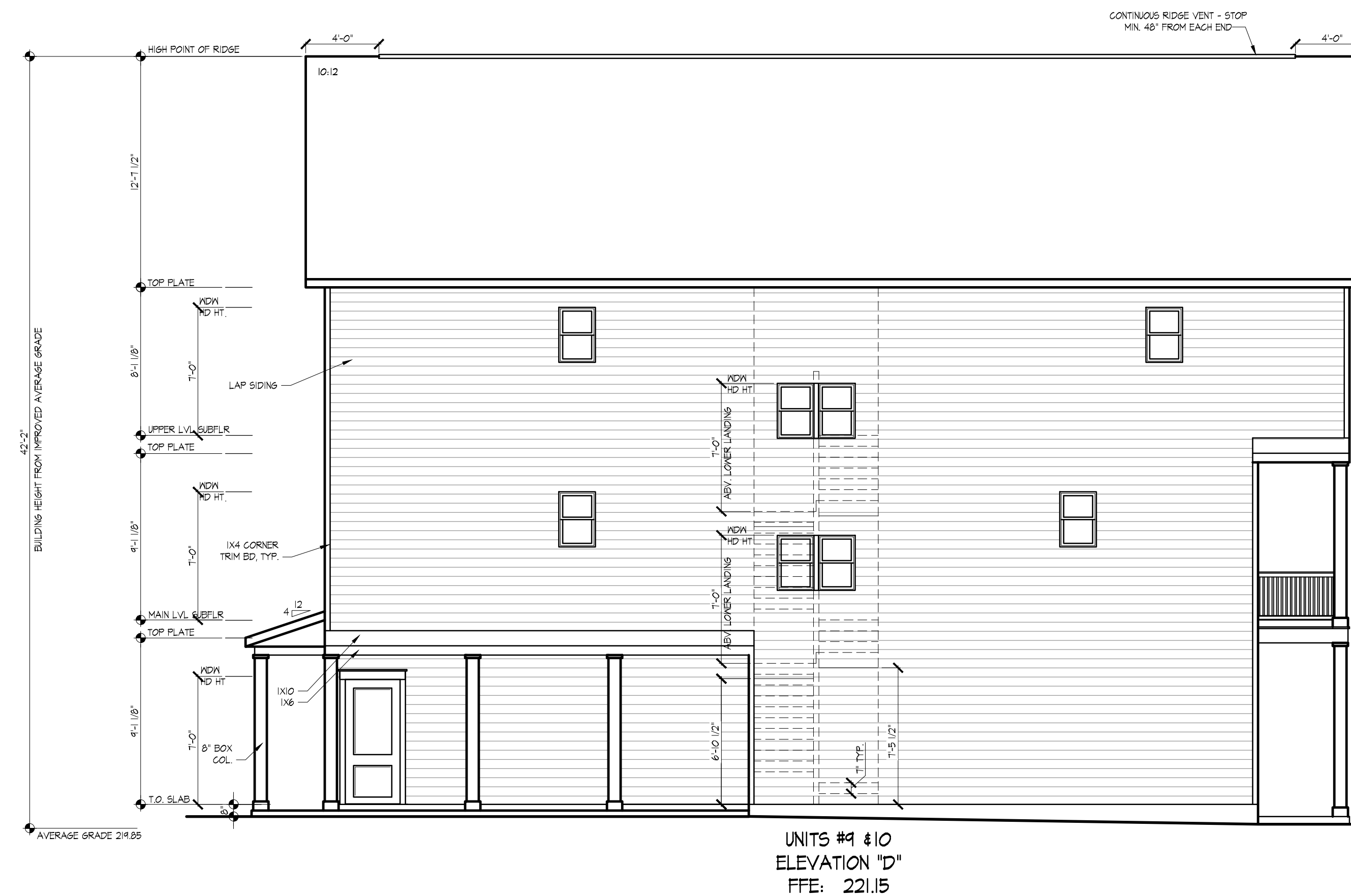
UNITS #9 #10 ELEVATION "D" FFE: 221.15 EDGEWATER COMMONS BUILDING N6 PLATTE RIVER DRIVE ELEVATION SCALE 3/16"=1'-0"
