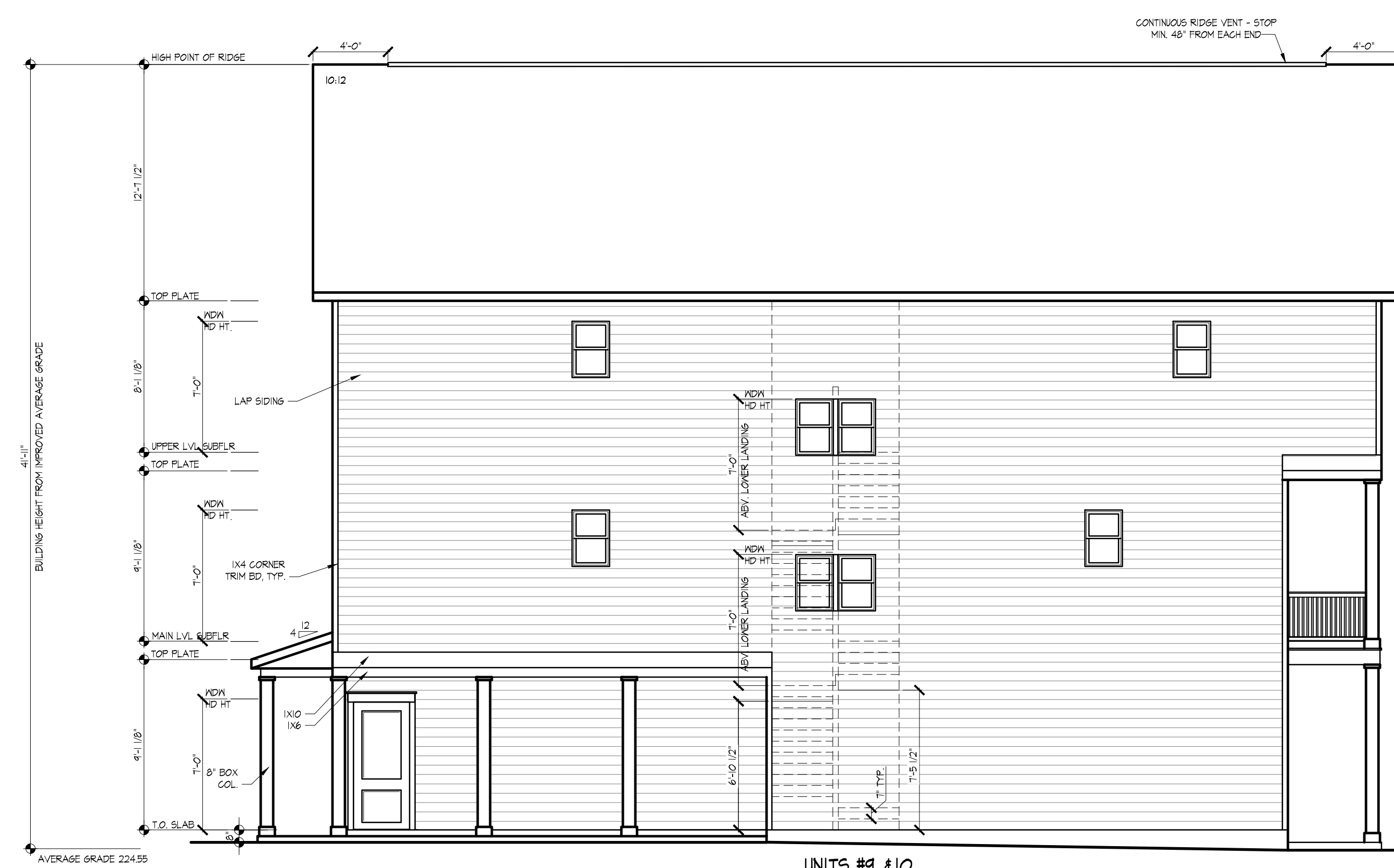
UNITS #9 #10 ELEVATION "D" FFE: 225.55 EDGEWATER COMMONS BUILDING N7 PLATTE RIVER DRIVE ELEVATION SCALE 3/16"=1'-0"
