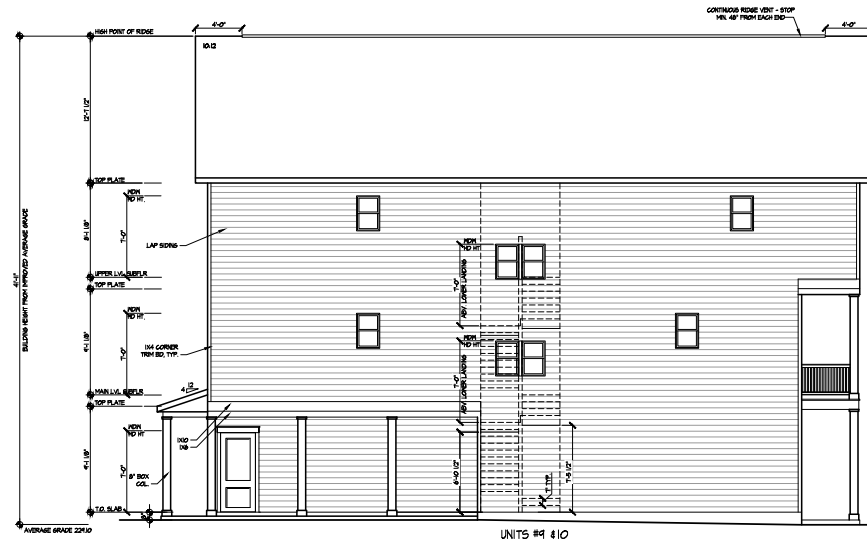
UNITS #1 & 10 ELEVATION "D" FFE: 230.15 EDGEWATER COMMONS BUILDING N8 PLATTE RIVER DRIVE ELEVATION SCALE 3/16"=1'-0"
