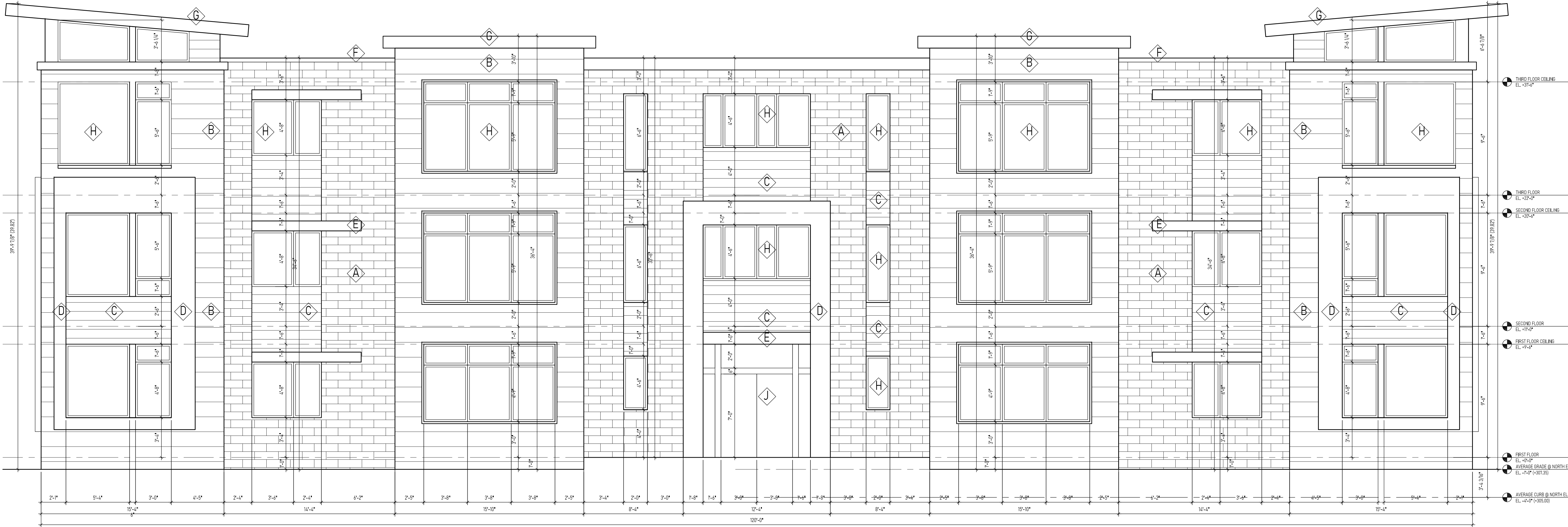
1 NORTH AND SOUTH EXTERIOR ELEVATION A2.1 SCALE - 1/4" = 1'-0"
