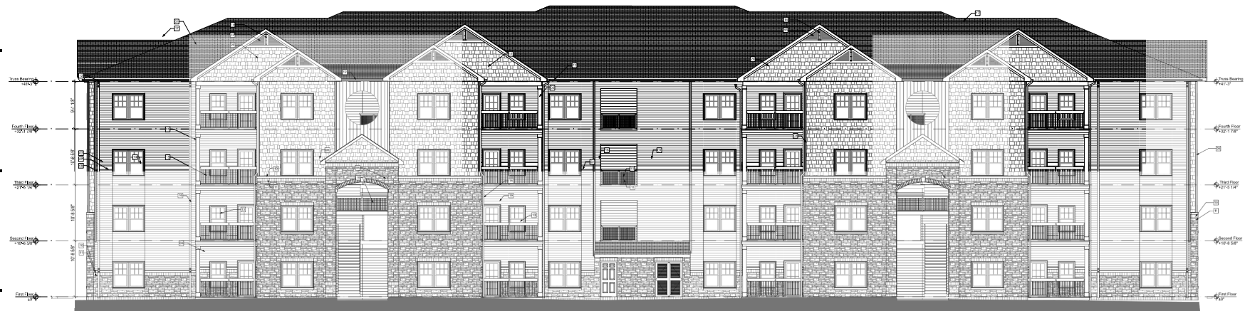
E1 BUILDING # 11 - FRONT ELEVATION SCALE: 1/8" = 1'-0"
