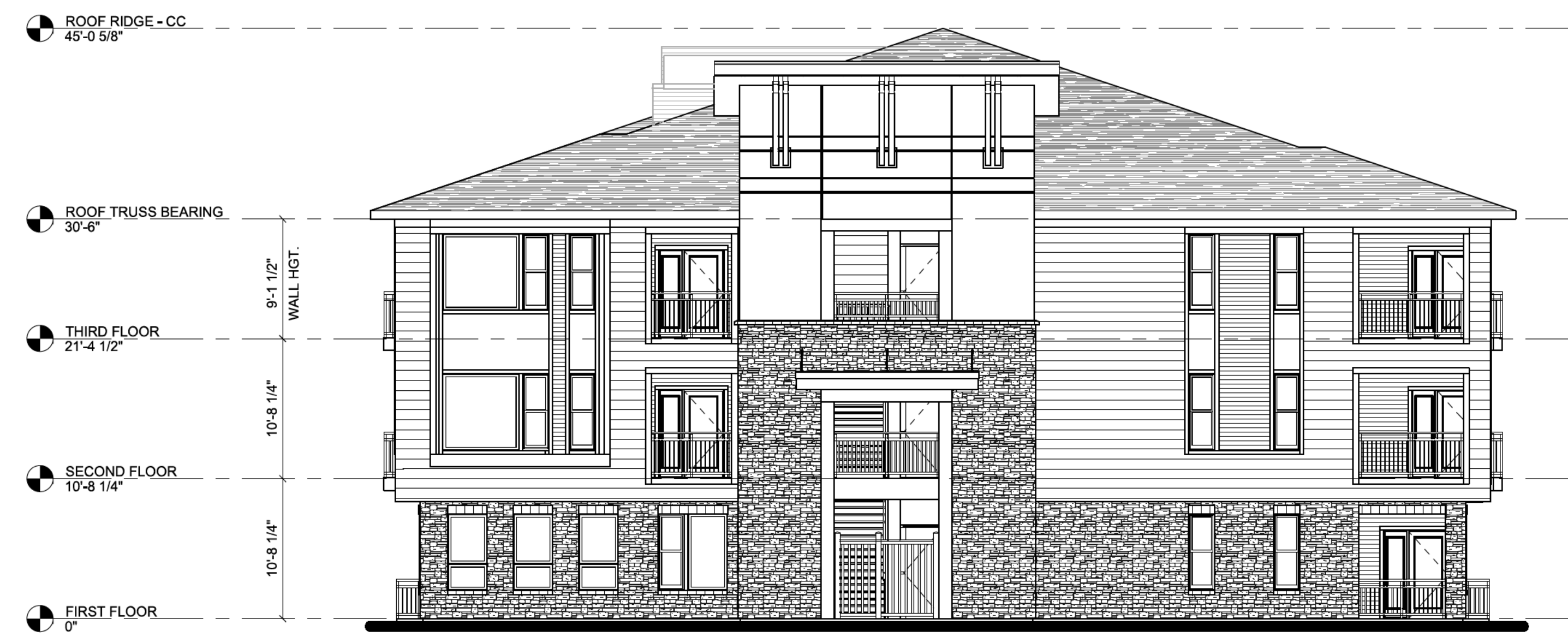
1 BUILDING TYPE C - EAST ENTRANCE ELEVATION
