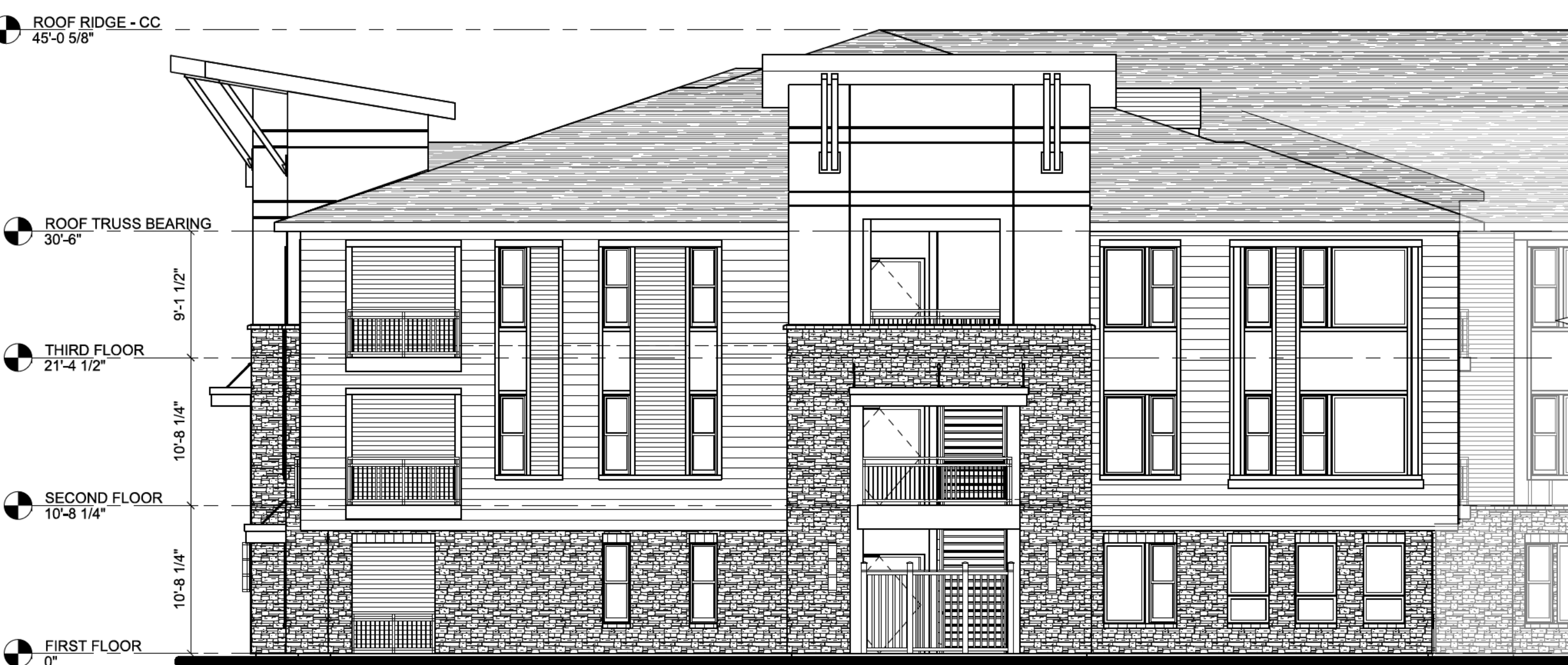
4 BUILDING TYPE A - EAST ENTRANCE ELEVATION
