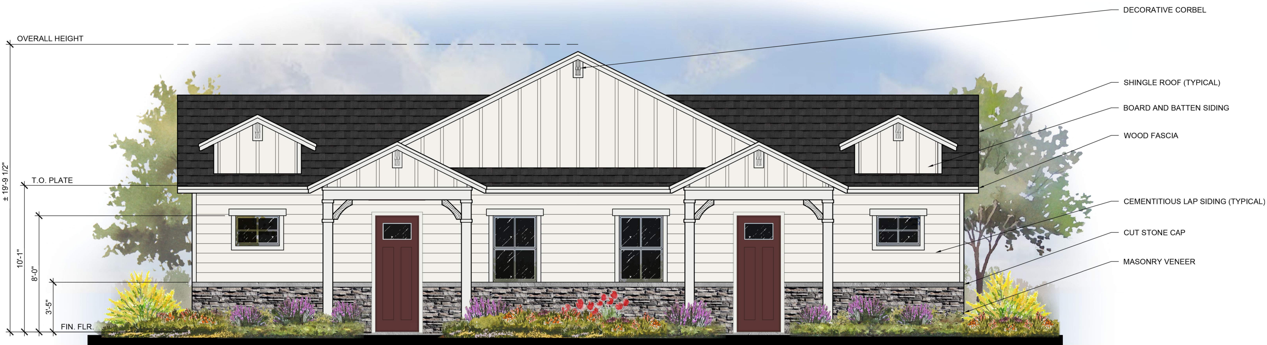
FRONT ELEVATION ELEVATION B - MODERN FARMHOUSE 1/4" = 1'-0"
