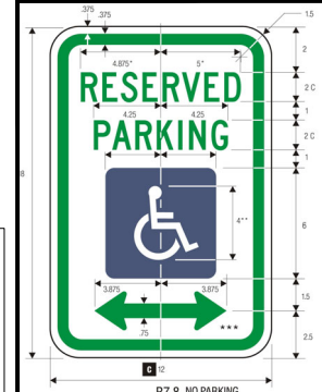
ACCESSIBLE PARKING SIGNAGE DETAIL N.T.S.
