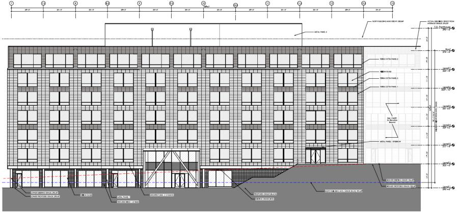
Building 1 - South Elevation 1 - Interior Courtyard Facing
