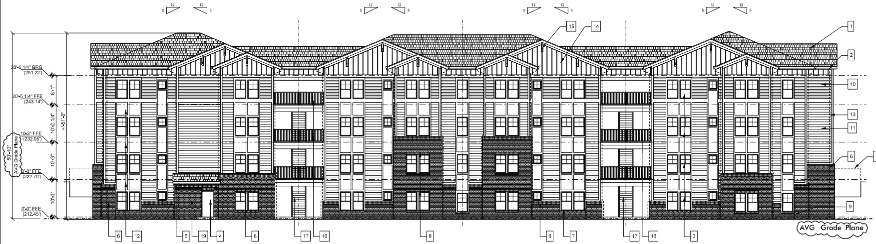
Elevation - REAR - Building No. 4 Scale: 1/8" = 1'-0"
