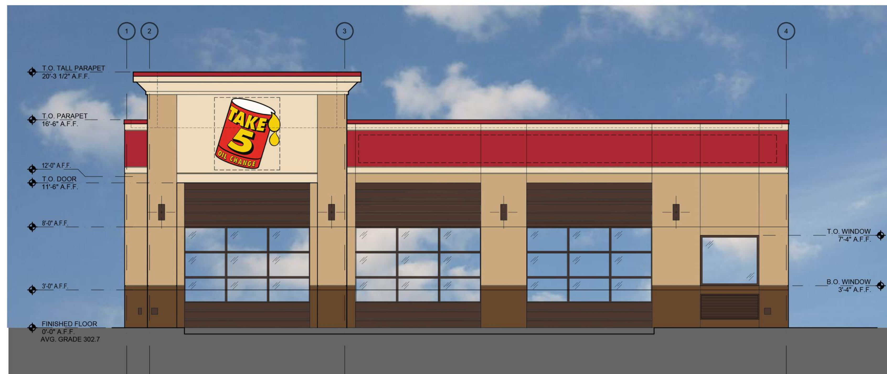
3 SOUTH ELEVATION - FACING NEW BERN AVE Scale: 1/4"=1'-0"
