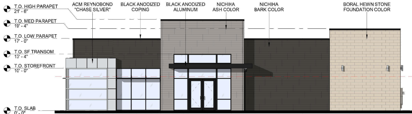
NORTHEAST ELEVATION (43%) STREET FACING
